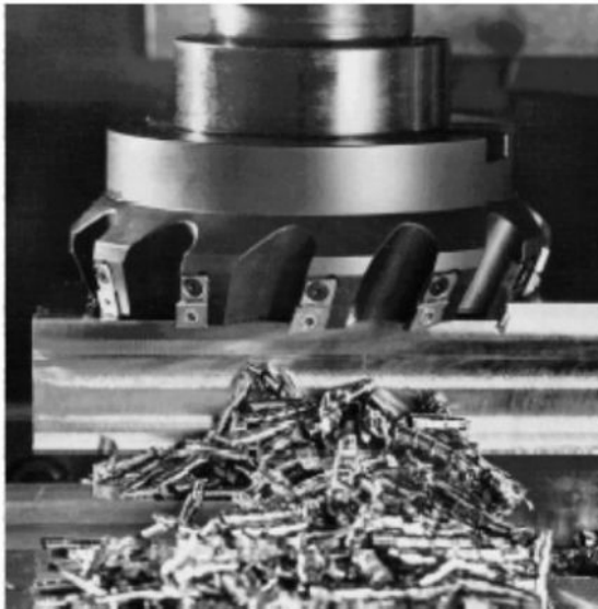
Fig:A face milling cutter with indexable inserts.
