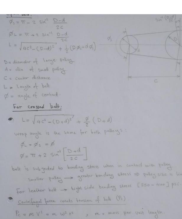
Smaller pulley -> greater benching stress => pulley size is limited.
