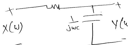
$$H(\omega) = \frac{Y(\omega)}{X(\omega)} = \frac{\frac{Y_{j\omega C}}{R + \frac{1}{j\omega C}}}{1 + j\omega CR} = \frac{1}{1 + j\omega CR}$$
