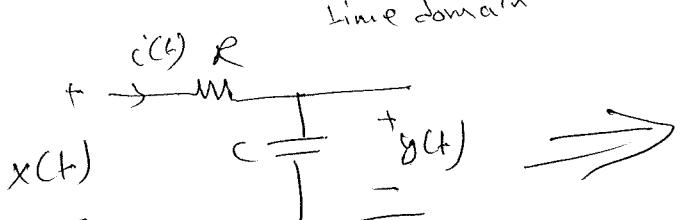
$$Y(\omega) = X(\omega) \left( \frac{\frac{1}{j\omega C}}{R + \frac{1}{j\omega C}} \right)$$
