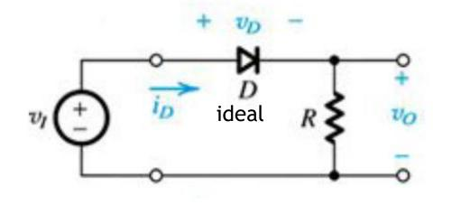
A) when  $V_i(t) > 0$ , Diode is on (short circuit)  $\therefore V_o(t) = V_i(t)$
