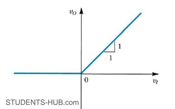
Design a diode circuit that have the given characteristic curve
