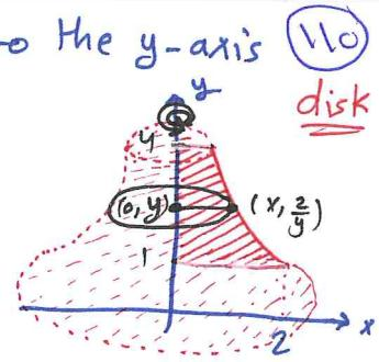
Example: Find the volume of the solid generated by revolving the region between the  $y$ -axis and the curve  $x = \frac{2}{y}$ ,  $1 \leq y \leq 4$  about the  $y$ -axis.
