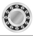
In the simplified sketch of a ball bearing shown, the diameter of the inner race A is 60 mm and the diameter of each ball is 12 mm. The outer race B is stationary while the inner race has an angular velocity of 3600 rpm. Determine (a) the speed of the center of each ball, (b) the angular velocity of each ball, (c) the number of times per minute each ball describes a complete circle.
