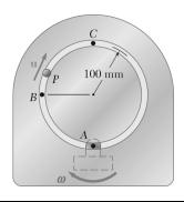
Pin P slides in a circular slot cut in the plate shown at a constant relative speed u = 90 mm/s. Knowing that at the instant shown the angular velocity  $\omega$  of the plate is 3 rad/s clockwise and is decreasing at the rate of 5 rad/s<sup>2</sup>, determine the acceleration of the pin if it is located at (a) Point A, (b) Point B, (c) Point C.
