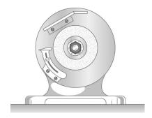
A small grinding wheel is attached to the shaft of an electric motor which has a rated speed of 3600 rpm. When the power is turned on, the unit reaches its rated speed in 5 s, and when the power is turned off, the unit coasts to rest in 70 s. Assuming uniformly accelerated motion, determine the number of revolutions that the motor executes (a) in reaching its rated speed, (b) in coasting to rest.
