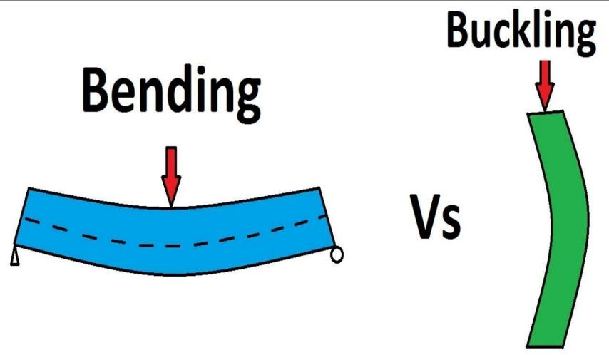
If you apply gradually increasing compressive forces at each end, very small axial deflections would happen at first, but then the stick would bend (buckle), and very quickly bend so much as to possibly fracture.
