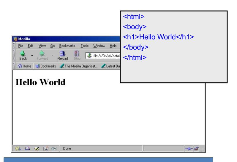
Applying a browser to catalog.xml (catalog.xml has a link to catalog.xsl)
