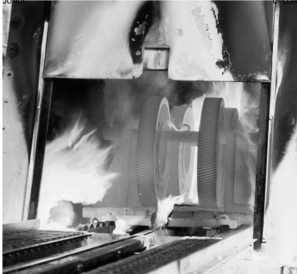
**Figure 5.1 Furnace for heat treating steel using the carburization process. (Courtesy of Cincinnati Steel Treating).**
