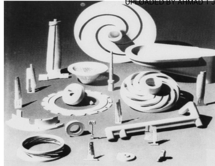
**Figure 1.6 A variety of complex ceramic components, including impellers and blades, which allow turbine engines to operate more efficiently at higher temperatures. (Courtesy of Certech, Inc.)**
