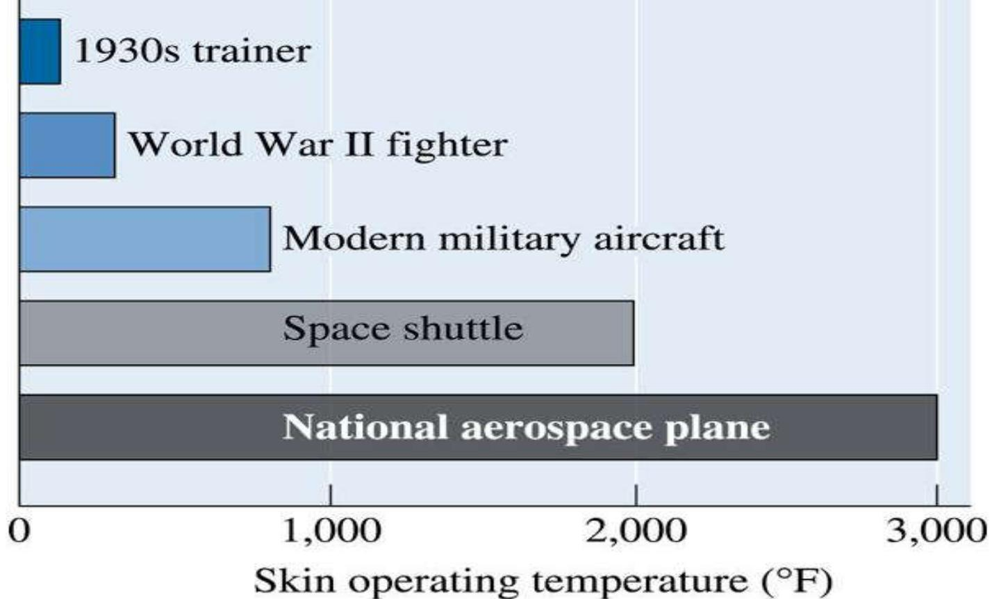
**Figure 1.13 Skin operating temperatures for aircraft have increased with the development of improved materials. (After M. Steinberg, Scientific American, October, 1986.)**
