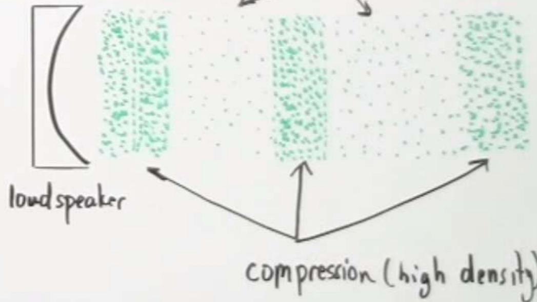
A vibrating loudspeaker alternately compresses and expands the air molecules in contact, producing a longitudinal wave.
