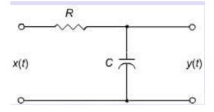
B. Find the 3-dB bandwidth of the circuit
