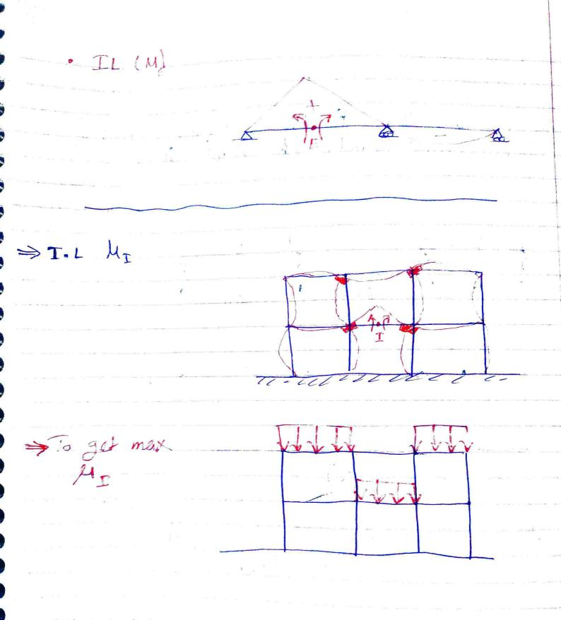
. Example: three 5 beam. · Draw qualitative IL for the Bending Homent of the beam, and develop the load cases. · Choose midspans & Interior supports . [ max Ma - load Cases · load Case (LCI) live load for may Ma Load Case (LG) Pormain Ma
