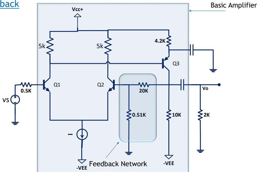
Negative FeedbackPractical configuration and the effect of loading2) Series - Shunt Feedback**Example:**
