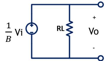
2) Shunt - Shunt Feedback
