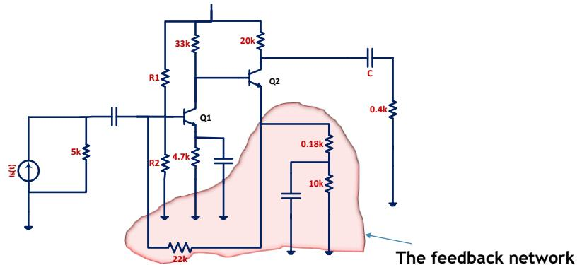
**New Basic Amplifier :**
