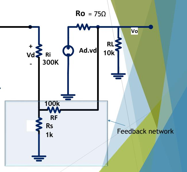
Negative FeedbackPractical configuration and the effect of loading2) Series - Shunt Feedback**Example: Non-Inverting Am****The Feed-Back Network:**
