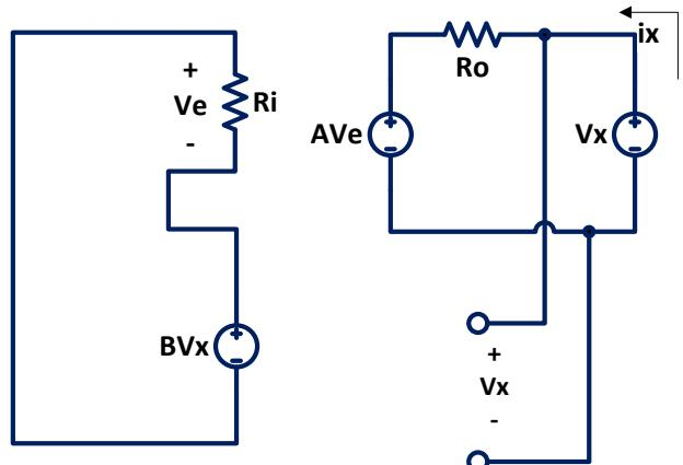
**Series Feedback at the input always raises the input impedance by  $(1+AB)$**
