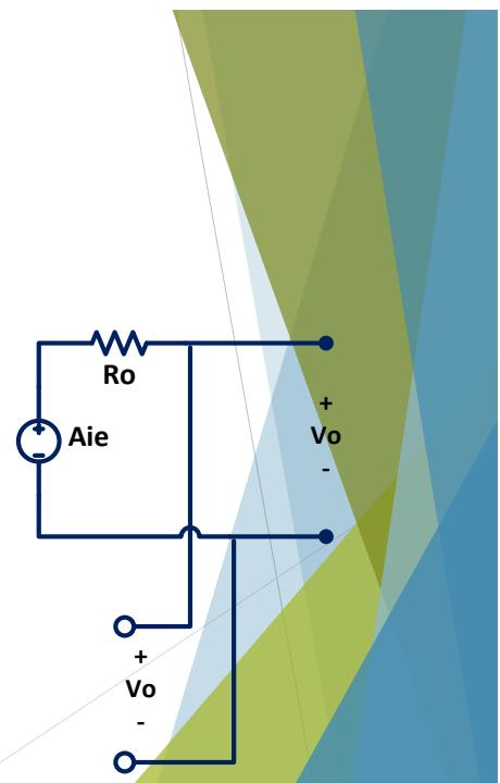
Negative Feedback2) Shunt - Shunt FeedbackEquivalent ckt of Shunt Shunt amplifierIf  $A \rightarrow \infty$  ;
