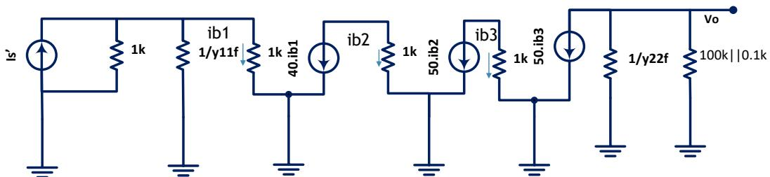
Negative FeedbackPractical configuration and the effect of loading1) Shunt - Shunt Feedback**The Feedback network**
