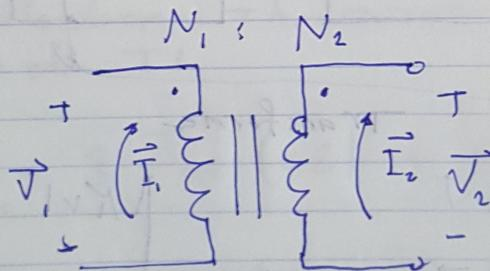
$$\frac{V_2}{V_1} = \frac{N_2}{N_1}, \quad \frac{I_2}{I_1} = \frac{N_1}{N_2}, \quad \frac{N_2}{N_1} = a$$
