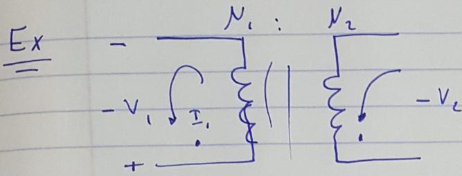
$$\frac{V_2}{V_1} = \frac{N_2}{N_1}, \quad \frac{I_2}{I_1} = -\frac{N_1}{N_2}$$
