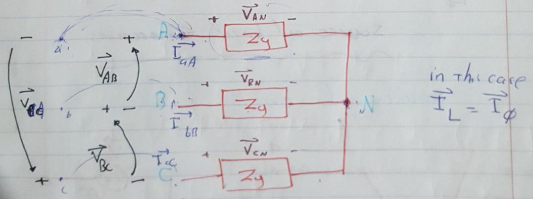
$\vec{V}_{AN}, \vec{V}_{BN}, \vec{V}_{CN}$  phase voltages on L-N voltages,
