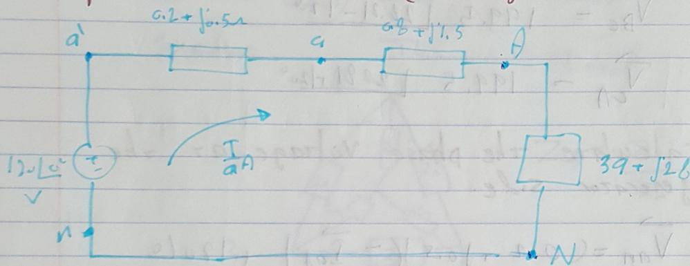
$$b) \vec{I}_{aA} = \frac{120 \angle 0^\circ}{(0.2 + j0.5) + (0.6 + j1.5) + (39 + j26)} = 2.4 \angle -36.87^\circ \text{ A}$$
