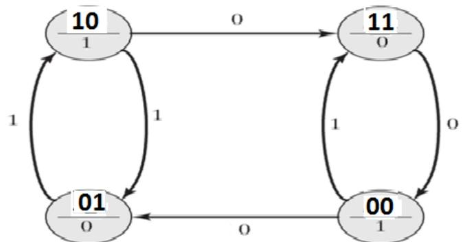
7. We would like to design a Moore sequential circuit that dynamically detects the occurrence of the sequence 1100 on a single external input X. The output of the circuit Y will be normally 0, going to 1 only when the full required sequence is detected. Give:
