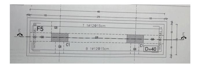
**Question 2**: The following drawing is a Longitudinal section in a beam using scale 1:20 draw section A-A(cross section). The depth and width of the beam are(25,60) cm respectively with (2 ø10)stirrups. Use appropriate layers and sheet size. (Note: dimensions are in cm)
