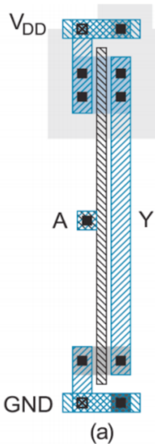
FIG 1.40 Inverter with dimensions labeled
