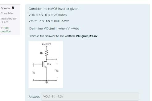
$$V_{I} = V_{DD} = 5 \text{ V} \Rightarrow V_{O} = V_{OL(m,n)}$$
