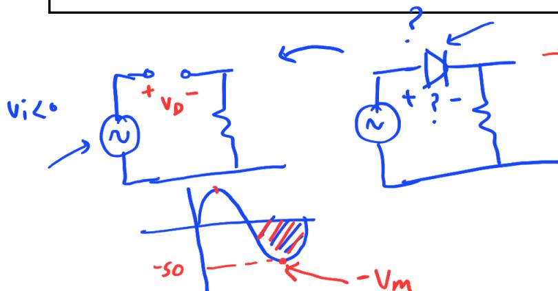
$\rightarrow$  We inspect what is the maximum reverse voltage that the diode will see in the given circuit
