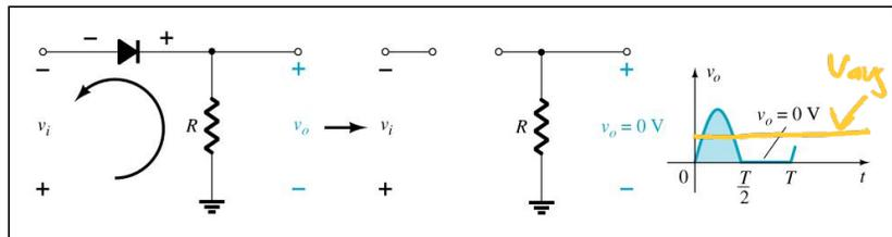
The diode conducts only when it is forward biased, therefore only half of the AC cycle passes through the diode to the output.
