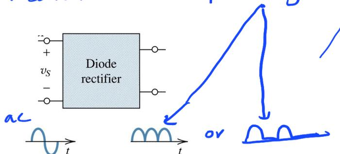
➤ Used to convert ac voltage (with zero average value) to pulsating dc voltage (non zero average)
