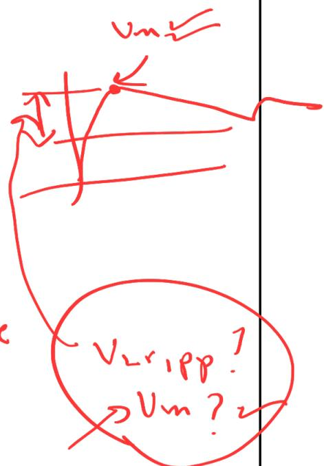
$\Rightarrow$  To Determine the ripple factor we need to find the peak to peak ripple  $V_{Lr,p-p}$
