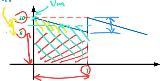
$$V_{O,DC} = V_{O,AVG} = \frac{1}{T} \int_0^T V_O(t) dt$$
