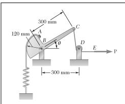
A force **P** of magnitude 240 N is applied to end E of cable CDE, which passes under pulley D and is attached to the mechanism at C. Neglecting the weight of the mechanism and the radius of the pulley, determine the value of  $\theta$  corresponding to equilibrium. The constant of the spring is k = 4 kN/m, and the spring is unstretched when  $\theta = 90^{\circ}$ .
