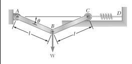
A vertical load **W** is applied to the linkage at B. The constant of the spring is k, and the spring is unstretched when AB and BC are horizontal. Neglecting the weight of the linkage, derive an equation in  $\theta$ , W, I, and k that must be satisfied when the linkage is in equilibrium.
