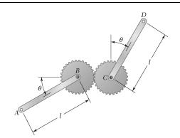
Two uniform rods, each of mass m, are attached to gears of equal radii as shown. Determine the positions of equilibrium of the system and state in each case whether the equilibrium is stable, unstable, or neutral.
