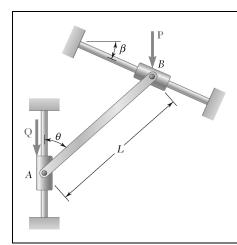
A slender rod AB is attached to two collars A and B that can move freely along the guide rods shown. Knowing that  $\beta = 30^{\circ}$ , P = 100 N, and Q = 25 N, determine the value of the angle  $\theta$  corresponding to equilibrium.
