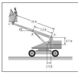
The telescoping arm ABC is used to provide an elevated platform for construction workers. The workers and the platform together weigh 500 lb and their combined center of gravity is located directly above C. For the position when  $\theta = 20^{\circ}$ , determine the force exerted on pin B by the single hydraulic cylinder BD.
