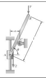
Determine the value of  $\theta$  corresponding to the equilibrium position of the rod of Problem 10.10 when l = 30 in., a = 5 in., P = 25 lb, and Q = 40 lb.
