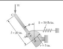
A load **W** of magnitude 100 lb is applied to the mechanism at C. Knowing that the spring is unstretched when  $\theta = 15^{\circ}$ , determine that value of  $\theta$  corresponding to equilibrium and check that the equilibrium is stable.
