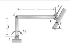
For the linkage shown, determine the force **Q** required for equilibrium when l = 18 in., M = 600 lb·in., and  $\theta = 70^{\circ}$ .
