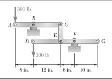
Determine the vertical force  $\mathbf{P}$  that must be applied at G to maintain the equilibrium of the linkage.
