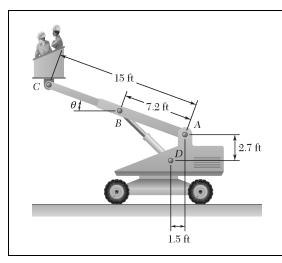
Solve Problem 10.45 assuming that the workers are lowered to a point near the ground so that  $\theta = -20^{\circ}$ .
