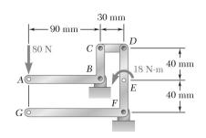
Determine the vertical force  $\mathbf{P}$  that must be applied at G to maintain the equilibrium of the linkage.
