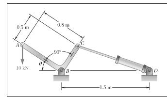
The position of member *ABC* is controlled by the hydraulic cylinder *CD*. For the loading shown, determine the force exerted by the hydraulic cylinder on pin *C* when  $\theta = 55^{\circ}$ .
