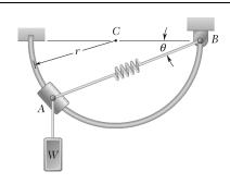
Collar A can slide freely on the semicircular rod shown. Knowing that the constant of the spring is k and that the unstretched length of the spring is equal to the radius r, determine the value of  $\theta$  corresponding to equilibrium when W = 50 lb, r = 9 in., and k = 15 lb/in.
