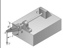
Using the method of Section 10.8, solve Problem 10.39. Determine whether the equilibrium is stable, unstable, or neutral. (*Hint:* The potential energy corresponding to the couple exerted by a torsion spring is  $\frac{1}{2}K\theta^2$ , where K is the torsional spring constant and  $\theta$  is the angle of twist.)
