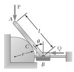
A slender rod of length l is attached to a collar at B and rests on a portion of a circular cylinder of radius r. Neglecting the effect of friction, determine the value of  $\theta$  corresponding to the equilibrium position of the mechanism when l = 200 mm, r = 60 mm, P = 40 N, and Q = 80 N.
