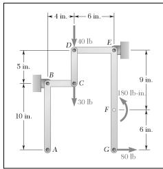
Determine the horizontal force  $\mathbf{P}$  that must be applied at A to maintain the equilibrium of the linkage.
