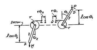
Left end of spring moves from a to b. Right end of spring moves from a' to b'. Elongation of spring
