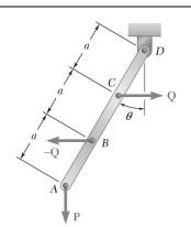
Rod AD is acted upon by a vertical force  $\mathbf{P}$  at end A, and by two equal and opposite horizontal forces of magnitude Q at points B and C. Derive an expression for the magnitude Q of the horizontal forces required for equilibrium.
