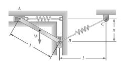
A slender rod AB, of weight W, is attached to two blocks A and B that can move freely in the guides shown. Knowing that both springs are unstretched when y=0, determine the value of y corresponding to equilibrium when W=80 N, l=550 mm, and k=600 N/m.
