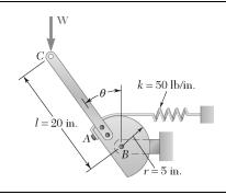
A load **W** of magnitude 100 lb is applied to the mechanism at C. Knowing that the spring is unstretched when  $\theta = 30^{\circ}$ , determine that value of  $\theta$  corresponding to equilibrium and check that the equilibrium is stable.
