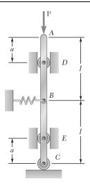
Two bars AB and BC are attached to a single spring of constant k that is unstretched when the bars are vertical. Determine the range of values of P for which the equilibrium of the system is stable in the position shown.
