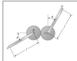
Two uniform rods, AB and CD, are attached to gears of equal radii as shown. Knowing that  $W_{AB} = 8$  lb and  $W_{CD} = 4$  lb, determine the positions of equilibrium of the system and state in each case whether the equilibrium is stable, unstable, or neutral.
