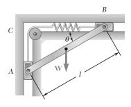
A slender rod AB, of weight W, is attached to two blocks A and B that can move freely in the guides shown. Knowing that the spring is unstretched when AB is horizontal, determine three values of  $\theta$  corresponding to equilibrium when W = 300 lb, l = 16 in., and k = 75 lb/in. State in each case whether the equilibrium is stable, unstable, or neutral.
