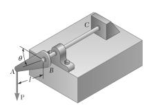
Solve Problem 10.39 assuming that P = 350 N, l = 250 mm, and  $K = 12.5 \text{ N} \cdot \text{m/rad}$ . Obtain answers in each of the following quadrants:  $0 < \theta < 90^{\circ}, 270^{\circ} < \theta < 360^{\circ}, 360^{\circ} < \theta < 450^{\circ}$ .
