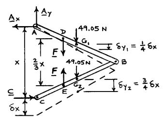
During the virtual displacement, Points D and E move apart a distance  $\delta(DE) = \frac{2}{3}\delta x$  and the total work done by the forces exerted at D and E is  $-F\left(\frac{2}{3}\delta x\right)$
