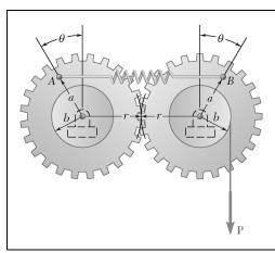
A spring AB of constant k is attached to two identical gears as shown. Knowing that the spring is undeformed when  $\theta = 0$ , determine two values of the angle  $\theta$  corresponding to equilibrium when P = 30 lb, a = 4 in., b = 3 in., r = 6 in., and k = 5 lb/in. State in each case whether the equilibrium is stable, unstable, or neutral.
