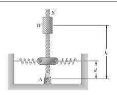
Rod AB is attached to a hinge at A and to two springs, each of constant k. If h = 45 in., k = 6 lb/in., and W = 60 lb, determine the smallest distance d for which the equilibrium of the rod is stable in the position shown. Each spring can act in either tension or compression.
