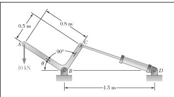
The position of member ABC is controlled by the hydraulic cylinder CD. Determine the angle  $\theta$ knowing that the hydraulic cylinder exerts a 15-kN force on pin C.
