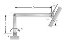
For the linkage shown, determine the couple M required for equilibrium when l=1.8 ft, Q=40 lb, and  $\theta=65^{\circ}$ .
