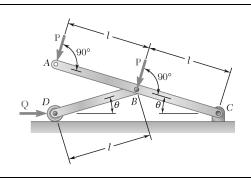
Derive an expression for the magnitude of the force  ${\bf Q}$  required to maintain the equilibrium of the mechanism shown.
