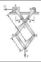
Knowing that the coefficient of static friction between the block attached to rod ACE and the horizontal surface is 0.15, determine the magnitude of the largest and smallest force  $\mathbf{Q}$  for which equilibrium is maintained when  $\theta = 30^{\circ}$ , l = 0.2 m, and P = 40 N.
