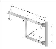
Determine the value of  $\theta$  corresponding to the equilibrium position of the mechanism of Problem 10.12 when P = 80 N and Q = 100 N.
