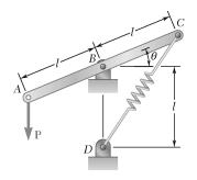
Knowing that the constant of spring CD is k and that the spring is unstretched when rod ABC is horizontal, determine the value of  $\theta$  corresponding to equilibrium for the data indicated.
