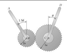
Two uniform rods, each of mass m and length l, are attached to gears as shown. For the range  $0 \le \theta \le 180^\circ$ , determine the positions of equilibrium of the system and state in each case whether the equilibrium is stable, unstable, or neutral.
