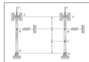
Two bars are attached to a single spring of constant k that is unstretched when the bars are vertical. Determine the range of values of P for which the equilibrium of the system is stable in the position shown.
