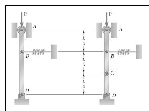
Two bars are attached to a single spring of constant k that is unstretched when the bars are vertical. Determine the range of values of P for which the equilibrium of the system is stable in the position shown.
