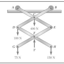
Determine the force P required to maintain the equilibrium of the linkage shown. All members are of the same length and the wheels at A and B roll freely on the horizontal rod.
