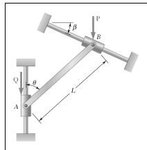
A slender rod AB is attached to two collars A and B that can move freely along the guide rods shown. Knowing that  $\beta = 30^{\circ}$  and P = Q = 400 N, determine the value of the angle  $\theta$  corresponding to equilibrium.
