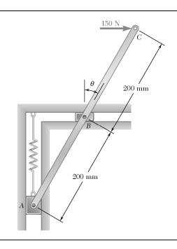
Rod ABC is attached to blocks A and B that can move freely in the guides shown. The constant of the spring attached at A is k=3 kN/m, and the spring is unstretched when the rod is vertical. For the loading shown, determine the value of  $\theta$  corresponding to equilibrium.
