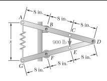
Two bars AD and DG are connected by a pin at D and by a spring AG. Knowing that the spring is 12 in. long when unstretched and that the constant of the spring is 125 lb/in., determine the value of x corresponding to equilibrium when a 900-lb load is applied at E as shown.
