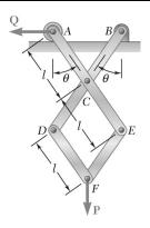
Determine the value of  $\theta$  corresponding to the equilibrium position of the mechanism of Prob. 10.14 when P = 270 N and Q = 960 N.
