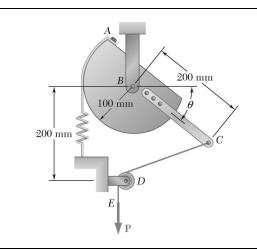
A vertical force **P** of magnitude 150 N is applied to end E of cable CDE, which passes over a small pulley D and is attached to the mechanism at C. The constant of the spring is k=4 kN/m, and the spring is unstretched when  $\theta=0$ . Neglecting the weight of the mechanism and the radius of the pulley, determine the value of  $\theta$  corresponding to equilibrium.
