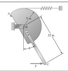
A horizontal force **P** of magnitude 40 lb is applied to the mechanism at C. The constant of the spring is k = 9 lb/in., and the spring is unstretched when  $\theta = 0$ . Neglecting the weight of the mechanism, determine the value of  $\theta$  corresponding to equilibrium.
