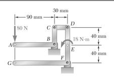
Determine the couple **M** that must be applied to member *DEFG* to maintain the equilibrium of the linkage.
