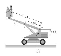
Referring to Problem 10.45 and using the value found for the force exerted by the hydraulic cylinder BD, determine the change in the length of BD required to raise the platform attached at C by 2.5 in.
