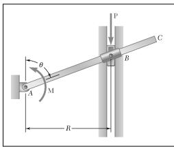
Collar B can slide along rod AC and is attached by a pin to a block that can slide in the vertical slot shown. Derive an expression for the magnitude of the couple M required to maintain equilibrium.
