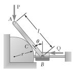
A slender rod of length l is attached to a collar at B and rests on a portion of a circular cylinder of radius r. Neglecting the effect of friction, determine the value of  $\theta$  corresponding to the equilibrium position of the mechanism when l = 14 in., r = 5 in., P = 75 lb, and Q = 150 lb.
