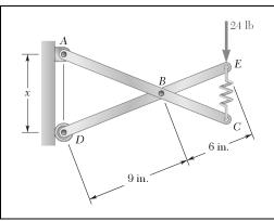
Two identical rods ABC and DBE are connected by a pin at B and by a spring CE. Knowing that the spring is 4 in. long when unstretched and that the constant of the spring is 8 lb/in., determine the distance x corresponding to equilibrium when a 24-lb load is applied at E as shown.
