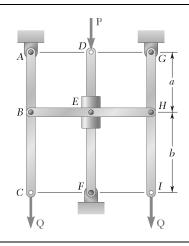
The horizontal bar *BEH* is connected to three vertical bars. The collar at E can slide freely on bar DF. Determine the range of values of Q for which the equilibrium of the system is stable in the position shown when a = 24 in., b = 20 in., and P = 150 lb.
