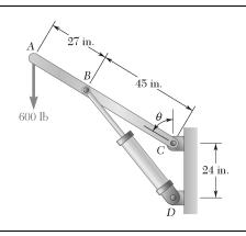
The position of boom ABC is controlled by the hydraulic cylinder BD. For the loading shown, (a) express the force exerted by the hydraulic cylinder on pin B as a function of the length BD, (b) determine the smallest possible value of the angle  $\theta$  if the maximum force that the cylinder can exert on pin B is 2.5 kips.
