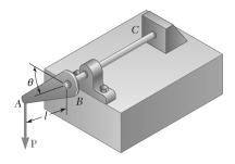
The lever AB is attached to the horizontal shaft BC that passes through a bearing and is welded to a fixed support at C. The torsional spring constant of the shaft BC is K; that is, a couple of magnitude K is required to rotate end B through 1 rad. Knowing that the shaft is untwisted when AB is horizontal, determine the value of  $\theta$  corresponding to the position of equilibrium when P = 100 N, l = 250 mm, and  $K = 12.5 \text{ N} \cdot \text{m/rad}$ .
