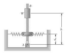
Rod AB is attached to a hinge at A and to two springs, each of constant k. If h = 25 in., d = 12 in., and W = 80 lb, determine the range of values of k for which the equilibrium of the rod is stable in the position shown. Each spring can act in either tension or compression.
