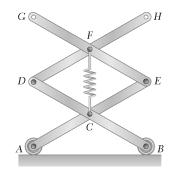
A spring of constant 15 kN/m connects Points C and F of the linkage shown. Neglecting the weight of the spring and linkage, determine the force in the spring and the vertical motion of Point G when a vertical downward 120-N force is applied (a) at Point C, (b) at Points C and H.
