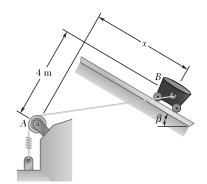
Cart B, which weighs 75 kN, rolls along a sloping track that forms an angle  $\beta$  with the horizontal. The spring constant is 5 kN/m, and the spring is unstretched when x = 0. Determine the distance x corresponding to equilibrium for the angle  $\beta$  indicated.
