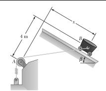
Cart B, which weighs 75 kN, rolls along a sloping track that forms an angle  $\beta$  with the horizontal. The spring constant is 5 kN/m, and the spring is unstretched when x = 0. Determine the distance x corresponding to equilibrium for the angle  $\beta$  indicated.
