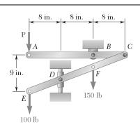
The two-bar linkage shown is supported by a pin and bracket at B and a collar at D that slides freely on a vertical rod. Determine the force  $\mathbf{P}$  required to maintain the equilibrium of the linkage.
