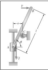
The slender rod AB is attached to a collar A and rests on a small wheel at C. Neglecting the radius of the wheel and the effect of friction, derive an expression for the magnitude of the force  $\mathbf{Q}$  required to maintain the equilibrium of the rod.
