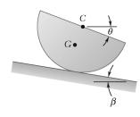
A homogeneous hemisphere of radius r is placed on an incline as shown. Assuming that friction is sufficient to prevent slipping between the hemisphere and the incline, determine the angle  $\theta$  corresponding to equilibrium when  $\beta = 10^{\circ}$ .
