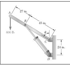
The position of boom ABC is controlled by the hydraulic cylinder BD. For the loading shown, determine the force exerted by the hydraulic cylinder on pin B when  $\theta = 65^{\circ}$ .
