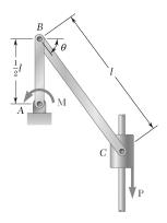
Knowing that the coefficient of static friction between collar C and the vertical rod is 0.40, determine the magnitude of the largest and smallest couple **M** for which equilibrium is maintained in the position shown, when  $\theta = 35^{\circ}$ , l = 600 mm, and P = 300 N.
