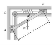
A slender rod AB, of weight W, is attached to two blocks A and B that can move freely in the guides shown. The constant of the spring is k, and the spring is unstretched when AB is horizontal. Neglecting the weight of the blocks, derive an equation in  $\theta$ , W, l, and k that must be satisfied when the rod is in equilibrium.
