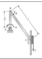
Denoting by  $\mu_s$  the coefficient of static friction between collar C and the vertical rod, derive an expression for the magnitude of the largest couple M for which equilibrium is maintained in the position shown. Explain what happens if  $\mu_s \ge \tan \theta$ .
