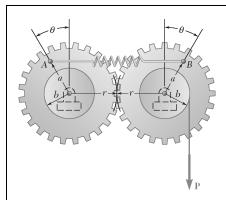
A spring AB of constant k is attached to two identical gears as shown. Knowing that the spring is undeformed when  $\theta = 0$ , and given that a = 60 mm, b = 45 mm, r = 90 mm, and k = 6 kN/m, determine (a) the range of values of P for which a position of equilibrium exists, (b) two values of  $\theta$  corresponding to equilibrium if the value of P is equal to half the upper limit of the range found in part a.
