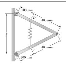
Two 5-kg bars AB and BC are connected by a pin at B and by a spring DE. Knowing that the spring is 150 mm long when unstretched and that the constant of the spring is 1 kN/m, determine the value of x corresponding to equilibrium.
