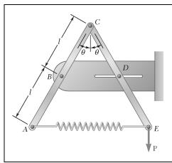
Two rods AC and CE are connected by a pin at C and by a spring AE. The constant of the spring is k, and the spring is unstretched when  $\theta = 30^{\circ}$ . For the loading shown, derive an equation in P,  $\theta$ , l, and k that must be satisfied when the system is in equilibrium.
