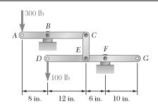
Determine the couple **M** that must be applied to member *DEFG* to maintain the equilibrium of the linkage.
