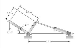
Referring to Problem 10.43 and using the value found for the force exerted by the hydraulic cylinder CD, determine the change in the length of CD required to raise the 10-kN load by 15 mm.
