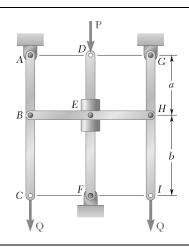
The horizontal bar BEH is connected to three vertical bars. The collar at E can slide freely on bar DF. Determine the range of values of P for which the equilibrium of the system is stable in the position shown when a = 150 mm, b = 200 mm, and Q = 45 N.
