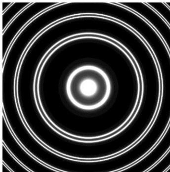
Fig. 8.7 The (computer generated) ring pattern as obtained (on the focal plane of a lens) in a Fabry-Perot etalon with n_f = 1 , h = 1.0 \text{ cm} and F = 400 , corresponding to \lambda_0 = 5000 \text{ \AA} ( = \lambda_1 ) and \lambda_0 = 4999.98 \text{ \AA} ( = \lambda_2 ).
