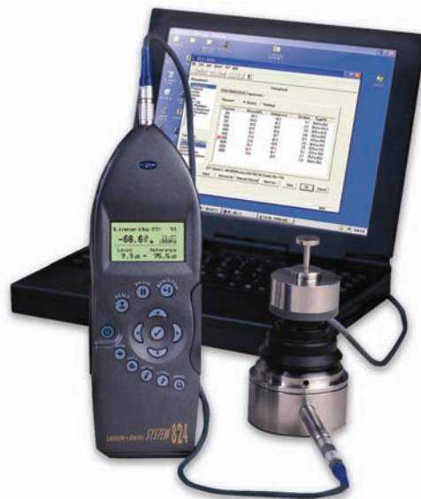
FIGURE 3.27 A commercial audiometer calibration device. A supra-aural earphone is placed on an artificial ear for calibration. A separate, smaller, artificial ear is used for calibration of insert receivers.
