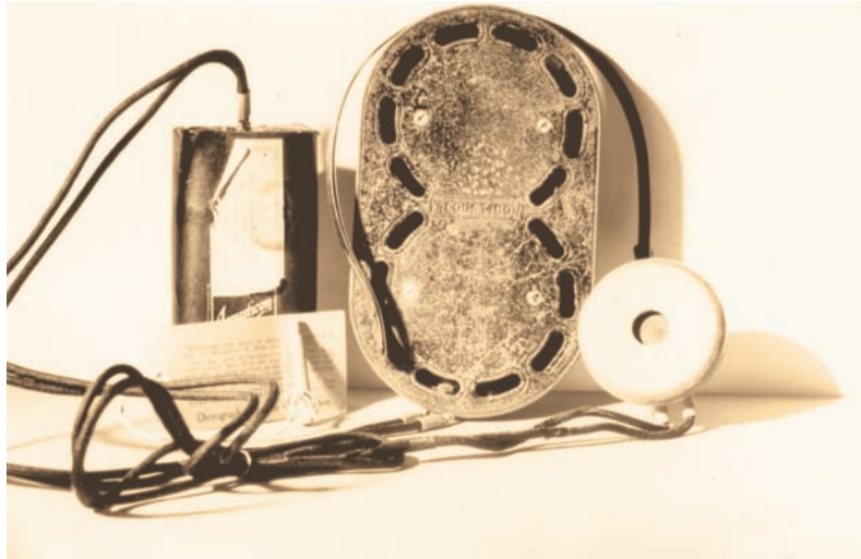
FIGURE 14.2 A complete carbon hearing aid consisting of a double carbon microphone for increased power, an earphone-style receiver with headband, and battery, circa 1910.
