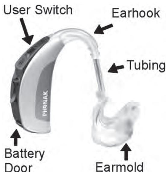
FIGURE 14-4. External features of a traditional BTE hearing aid with tubing and earmold attached. Source: Photo courtesy of Phonak, LLC and Westone® The In-Ear Experts®.
