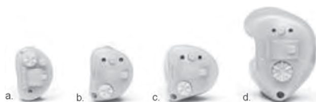
FIGURE 14-7. Four examples of traditional custom hearing aids ranging in size from ITC to full-sized ITE. Source: From Mueller, Ricketts, & Bentler, 2014, p. 256. Copyright 2014 by Plural Publishing, Inc.
