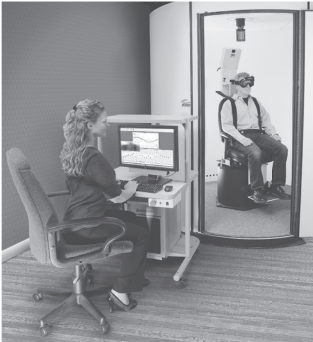
FIGURE 16-11. Illustration of a typical rotary chair testing arrangement. Source: Photo courtesy of Micromedical Technologies, 10 Kemp Drive, Chatham, IL 62629.
