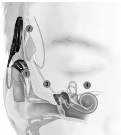
FIGURE 15-5. Cochlear implant with placement of external and internal CI components. (1) The microphone on the sound processor picks up and converts the sound into digital information. (2) This information is transferred through the coil to the implant located under the skin. (3) The implant sends electrical signals down the electrode into the cochlea. (4) The auditory nerve fibers in the cochlea pick up the electrical signals and conduct them up the auditory pathway to the auditory cortex. Source: Image courtesy of Cochlear Americas, © 2017.
