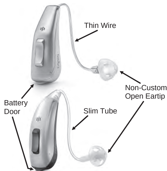
FIGURE 14-5. Two examples of mini-BTE hearing aids. The upper instrument is an RIC, and the lower instrument is an RITA configuration. Source: Photos courtesy of Sivantos GmbH.
