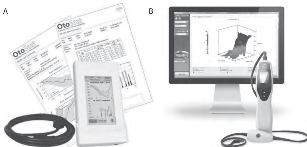
FIGURE 10–16. Wideband acoustic immittance (WAI) devices. A. Mimosa Acoustics Model OtoStat is a device that measures WAI at ambient pressure and reports in reflectance or absorbance at frequencies from 256 to 6000 Hz. B. Interacoustics Model Titan is a wideband tympanometer that measures the acoustic energy absorbed into the middle ear as a function of both frequency (from 226 to 8000 Hz) and pressure. As shown on the monitor, it uses those measurements to create a 3D graph of the absorbance where the audiologist can compare results from absorbance measurements to various pathologies. Source: Photos courtesy of Mimosa Acoustics (A) and Interacoustics (B).
