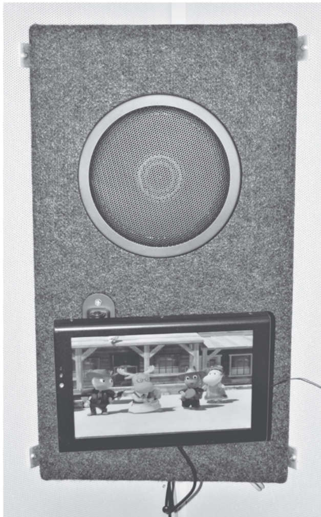
FIGURE 6-11. A sound-field speaker and a flat screen for projecting visual images when performing visual reinforcement audiometry (VRA). The VRA device allows the audiologist to pair the sound with the response when the child looks toward the speaker.
