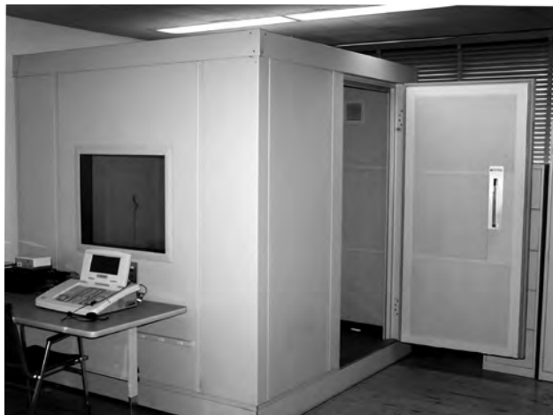
FIGURE 6-9. A single-room audiometric test environment. The patient sits inside the room and the tester and equipment are outside the room. The tester's equipment is connected to the room through a connector (jack) panel, and there is a window to maintain visual contact. In many clinics, the tester is also in another similarly treated test room that is connected to the patient's test booth, called a double-room test environment.
