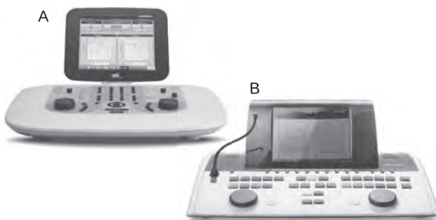
FIGURE 6-1. A and B. Some examples of two-channel diagnostic audiometers used for comprehensive clinical evaluations. A. Grason-Stadler Inc. Model AudioStar Pro. B. Interacoustic Model AC40. Source: Photos courtesy of Grason-Stadler Inc. ( A ) and Interacoustics ( B ).
