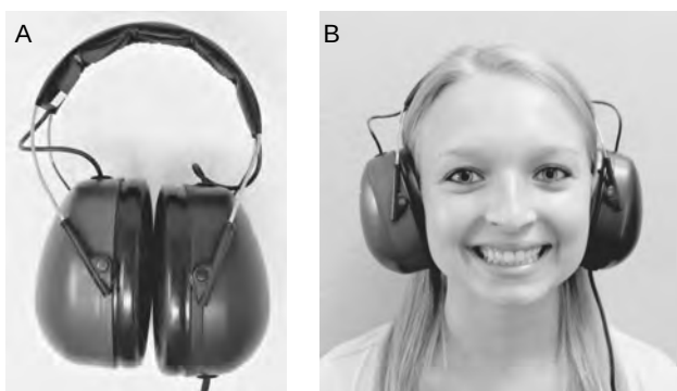
FIGURE 6–5. A. A set of extended high-frequency earphones (Sennheiser HDA200). B. Extended high-frequency earphones properly placed for testing.
