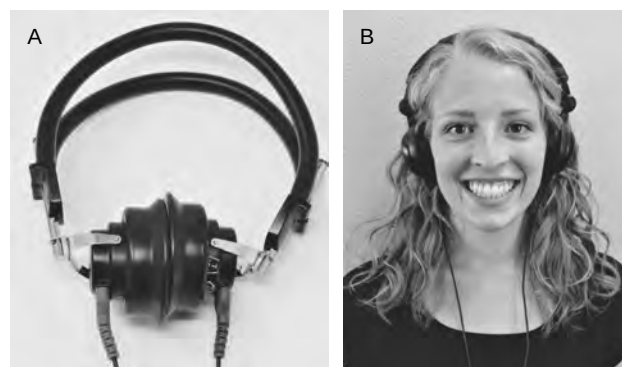
FIGURE 6-4. A. A set of supra-aural earphones (TDH-39). B. Supra-aural earphones properly placed for testing.
