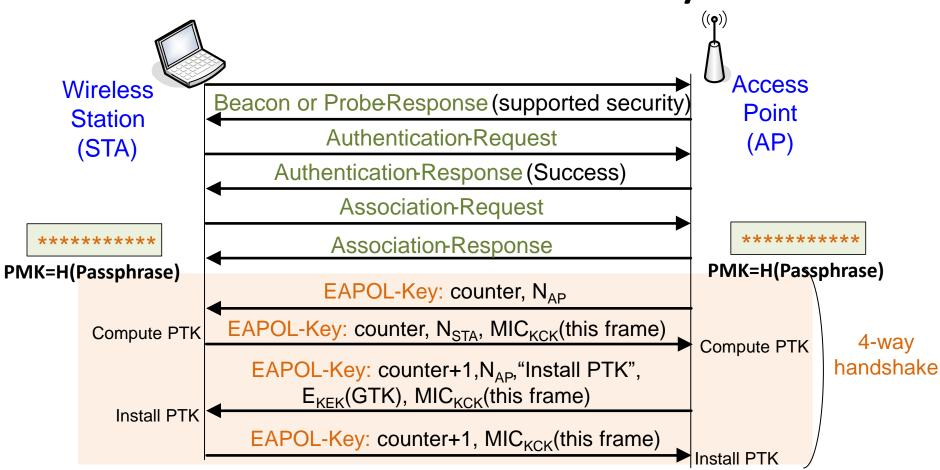
PMK = key derived from Passphrase /802.1x auth counter = replay prevention, reset for new PMK PRF = pseudo-random function PTK = PRF(PMK,MACaddr<sub>AP</sub>,MACaddr<sub>STA</sub>,N<sub>AP</sub>,N<sub>STA</sub>) KCK, KEK = parts of PTK STUDE MICS = message integrity check, a MAC
