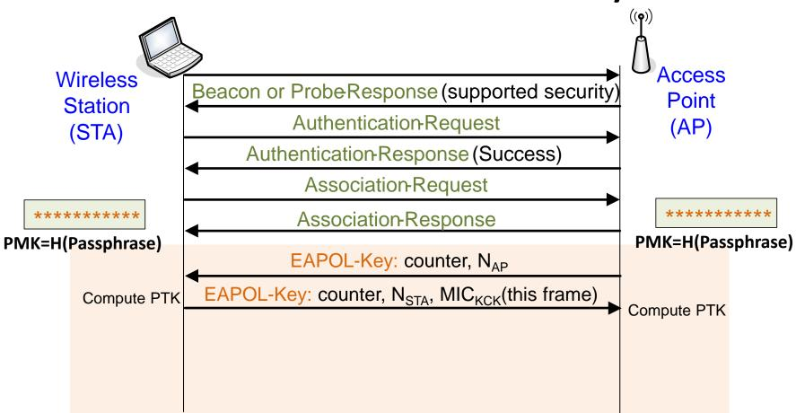
PMK = key derived from Passphrase/802.1x auth counter = replay prevention, reset for new PMK PRF = pseudo-random function PTK = PRF(PMK,MACaddr<sub>AP</sub>,MACaddr<sub>STA</sub>,N<sub>AP</sub>,N<sub>STA</sub>) KCK, KEK = parts of PTK STUDE MCS = message integrity check, a MAC
