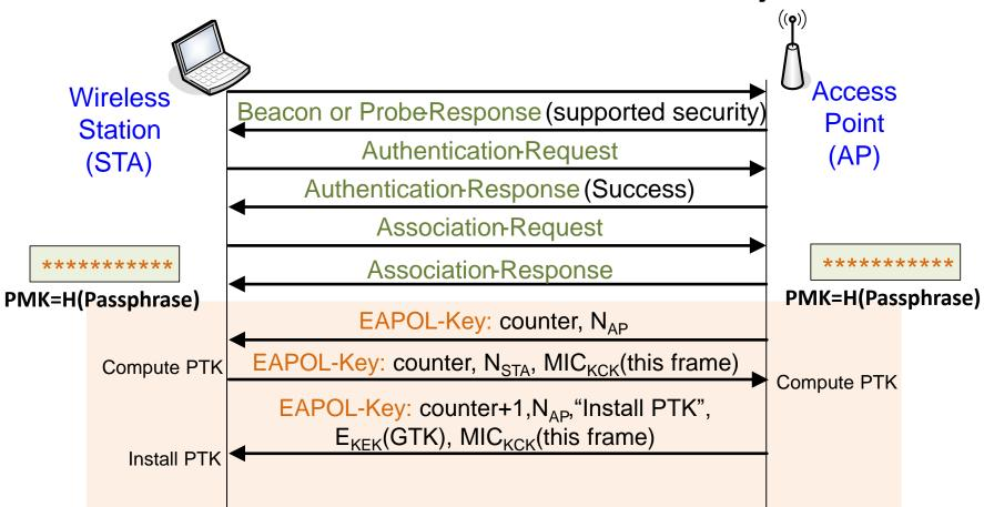
PMK = key derived from Passphrase/802.1x auth counter = replay prevention, reset for new PMK PRF = pseudo-random function PTK = PRF(PMK,MACaddr<sub>AP</sub>,MACaddr<sub>STA</sub>,N<sub>AP</sub>,N<sub>STA</sub>) KCK, KEK = parts of PTK STUDE MICS = message integrity check, a MAC
