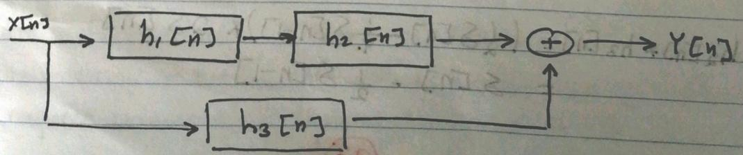
**Exercise:** Determine the overall impulse response of the following system, where the impulse responses of the components systems are:
