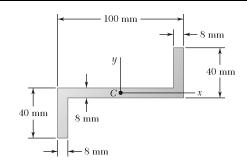
Using Mohr's circle, determine the moments of inertia and the product of inertia of the area of Problem 9.75 with respect to new centroidal axes obtained by rotating the x and y axes  $45^{\circ}$  clockwise.
