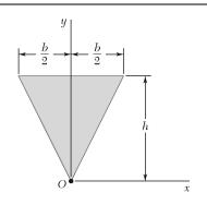
Determine the polar moment of inertia and the polar radius of gyration of the isosceles triangle shown with respect to Point *O*.
