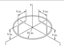
For the wire figure of Problem 9.146, determine the mass moment of inertia of the figure with respect to the axis through the origin characterized by the unit vector  $\lambda = (-3\mathbf{i} - 6\mathbf{j} + 2\mathbf{k})/7$ .
