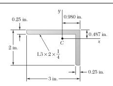
Using the parallel-axis theorem, determine the product of inertia of the area shown with respect to the centroidal x and y axes.
