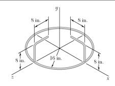
Aluminum wire with a weight per unit length of 0.033 lb/ft is used to form the circle and the straight members of the figure shown. Determine the mass moment of inertia of the assembly with respect to each of the coordinate axes.
