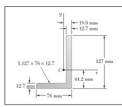
Using the parallel-axis theorem, determine the product of inertia of the area shown with respect to the centroidal x and y axes.
