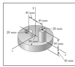
Shown is the machine element of Problem 9.141. Determine its mass moment of inertia with respect to the line joining the origin O and Point A.
