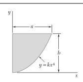
Determine by direct integration the moment of inertia of the shaded area with respect to the x axis.
