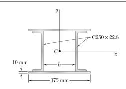
Two channels and two plates are used to form the column section shown. For b = 200 mm, determine the moments of inertia and the radii of gyration of the combined section with respect to the centroidal x and y axes.
