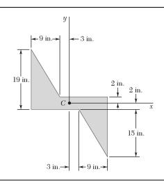
Using Mohr's circle, determine for the area indicated the orientation of the principal centroidal axes and the corresponding values of the moments of inertia.
