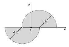
Using Mohr's circle, determine for the area indicated the orientation of the principal centroidal axes and the corresponding values of the moments of inertia.
