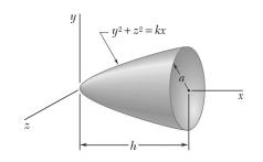
Determine by direct integration the mass moment of inertia with respect to the y axis of the paraboloid shown, assuming that it has a uniform density and a mass m.
