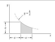
Determine by direct integration the moments of inertia of the shaded area with respect to the *x* and *y* axes.
