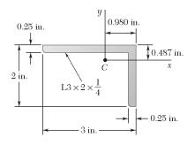
Determine the moments of inertia and the product of inertia of the  $L3 \times 2 \times \frac{1}{4}$ -in. angle cross section of Problem 9.74 with respect to new centroidal axes obtained by rotating the x and y axes  $30^{\circ}$ clockwise.
