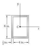
Two L6  $\times$  4  $\times$   $\frac{1}{2}$  -in. angles are welded together to form the section shown. Determine the moments of inertia and the radii of gyration of the combined section with respect to the centroidal x and y axes.
