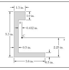
Using Mohr's circle, determine for the area indicated the orientation of the principal centroidal axes and the corresponding values of the moments of inertia.
