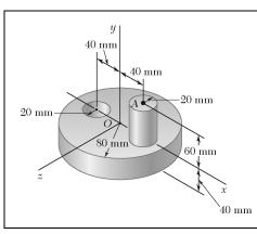
For the component described in Problem 9.165, determine (a) the principal mass moments of inertia at the origin, (b) the principal axes of inertia at the origin. Sketch the body and show the orientation of the principal axes of inertia relative to the x, y, and z axes.
