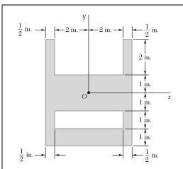
Determine the moment of inertia and the radius of gyration of the shaded area with respect to the *x* axis.
