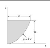
Determine by direct integration the moment of inertia of the shaded area with respect to the *y* axis.
