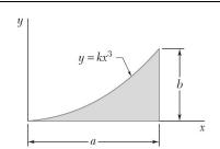
Determine by direct integration the product of inertia of the given area with respect to the *x* and *y* axes.
