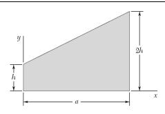
The area shown is revolved about the x axis to form a homogeneous solid of revolution of mass m. Using direct integration, express the mass moment of inertia of the solid with respect to the x axis in terms of m and h.
