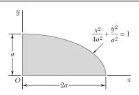
For the quarter ellipse of Problem 9.67, determine the orientation of the principal axes at the origin and the corresponding values of the moments of inertia.
