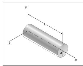
Determine by direct integration the mass moment of inertia with respect to the z axis of the right circular cylinder shown, assuming that it has a uniform density and a mass m.
