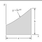
Determine by direct integration the moment of inertia of the shaded area with respect to the y axis.
