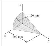
A subassembly for a model airplane is fabricated from three pieces of 1.5-mm plywood. Neglecting the mass of the adhesive used to assemble the three pieces, determine the mass moment of inertia of the subassembly with respect to each of the coordinate axes. (The density of the plywood is 780 kg/m<sup>3</sup>.)
