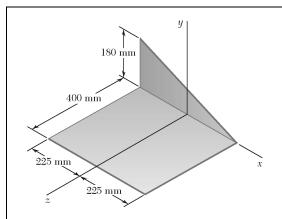
A section of sheet steel 2 mm thick is cut and bent into the machine component shown. Knowing that the density of steel is 7850 kg/m<sup>3</sup>, determine the mass products of inertia  $I_{xy}$ ,  $I_{yz}$ , and  $I_{zx}$  of the component.
