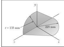
A section of sheet steel 2 mm thick is cut and bent into the machine component shown. Knowing that the density of steel is 7850 kg/m<sup>3</sup>, determine the mass products of inertia  $I_{xy}$ ,  $I_{yz}$ , and  $I_{zx}$  of the component.
