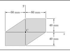
Using Mohr's circle, determine for the area indicated the orientation of the principal centroidal axes and the corresponding values of the moments of inertia.
