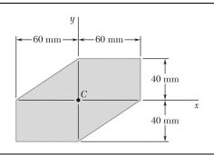
Determine the moments of inertia and the product of inertia of the area of Problem 9.72 with respect to new centroidal axes obtained by rotating the x and y axes 30° counterclockwise.
