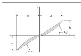
Determine the moment of inertia and the radius of gyration of the shaded area shown with respect to the *y* axis.
