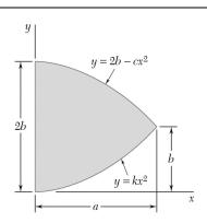
Determine the moment of inertia and the radius of gyration of the shaded area shown with respect to the y axis.
