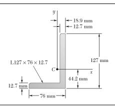
Using Mohr's circle, determine the moments of inertia and the product of inertia of the  $L127 \times 76 \times 12.7$ -mm angle cross section of Problem 9.78 with respect to new centroidal axes obtained by rotating the x and y axes  $45^{\circ}$  counterclockwise.
