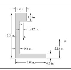
Using the parallel-axis theorem, determine the product of inertia of the area shown with respect to the centroidal x and y axes.
