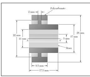
Shown is the cross section of a molded flat-belt pulley. Determine its mass moment of inertia and its radius of gyration with respect to the axis AA'. (The density of brass is  $8650 \text{ kg/m}^3$  and the density of the fiber-reinforced polycarbonate used is  $1250 \text{ kg/m}^3$ .)
