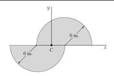
For the area indicated, determine the orientation of the principal axes at the origin and the corresponding values of the moments of inertia.
