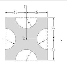
Determine the moments of inertia of the shaded area shown with respect to the x and y axes when a = 20 mm.
