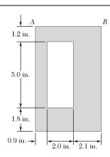
Determine the moments of inertia  $\overline{I}_x$  and  $\overline{I}_y$  of the area shown with respect to centroidal axes respectively parallel and perpendicular to side AB.
