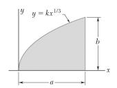
Determine by direct integration the moment of inertia of the shaded area with respect to the *y* axis.
