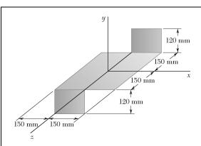
A 2-mm thick piece of sheet steel is cut and bent into the machine component shown. Knowing that the density of steel is 7850 kg/m<sup>3</sup>, determine the mass moment of inertia of the component with respect to each of the coordinate axes.
