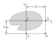
The shaded area is equal to 50 in<sup>2</sup>. Determine its centroidal moments of inertia  $\overline{I}_x$  and  $\overline{I}_y$ , knowing that  $\overline{I}_y = 2\overline{I}_x$  and that the polar moment of inertia of the area about Point A is  $J_A = 2250$  in<sup>4</sup>.
