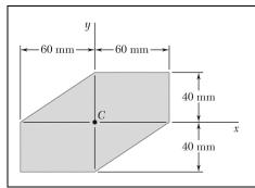
Using Mohr's circle, determine the moments of inertia and the product of inertia of the area of Problem 9.72 with respect to new centroidal axes obtained by rotating the x and y axes  $30^{\circ}$  counterclockwise.
