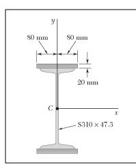
Two 20-mm steel plates are welded to a rolled S section as shown. Determine the moments of inertia and the radii of gyration of the combined section with respect to the centroidal x and y axes.
