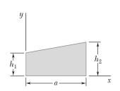
Determine by direct integration the moment of inertia of the shaded area with respect to the *x* axis.
