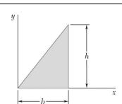
Determine by direct integration the product of inertia of the given area with respect to the x and y axes.
