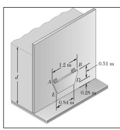
A vertical trapezoidal gate that is used as an automatic valve is held shut by two springs attached to hinges located along edge AB. Knowing that each spring exerts a couple of magnitude 1470 N  $\cdot$  m, determine the depth d of water for which the gate will open.
