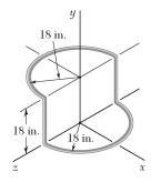
For the wire figure of Problem 9.147, determine the mass moment of inertia of the figure with respect to the axis through the origin characterized by the unit vector  $\lambda = (-3i - 6j + 2k)/7$ .
