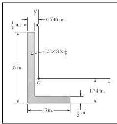
For the L5  $\times$  3  $\times$   $\frac{1}{2}$ -in. angle cross section shown, use Mohr's circle to determine (a) the moments of inertia and the product of inertia with respect to new centroidal axes obtained by rotating the x and y axes 30° clockwise, (b) the orientation of the principal axes through the centroid and the corresponding values of the moments of inertia.
