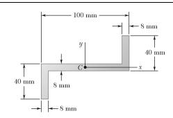
Determine the moments of inertia and the product of inertia of the area of Problem 9.75 with respect to new centroidal axes obtained by rotating the x and y axes  $45^{\circ}$  clockwise.
