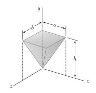
Determine by direct integration the mass moment of inertia with respect to the x axis of the pyramid shown, assuming that it has a uniform density and a mass m.
