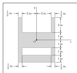
Determine the moment of inertia and the radius of gyration of the shaded area with respect to the *y* axis.
