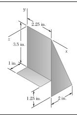
A framing anchor is formed of 0.05-in.-thick galvanized steel. Determine the mass moment of inertia of the anchor with respect to each of the coordinate axes. (The specific weight of galvanized steel is 470 lb/ft<sup>3</sup>.)
