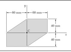
For the area indicated, determine the orientation of the principal axes at the origin and the corresponding values of the moments of inertia.
