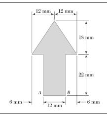
Determine the moments of inertia  $\overline{I}_x$  and  $\overline{I}_y$  of the area shown with respect to centroidal axes respectively parallel and perpendicular to side AB.
