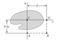
The polar moments of inertia of the shaded area with respect to Points A, B, and D are, respectively,  $J_A = 2880 \text{ in}^4$ ,  $J_B = 6720 \text{ in}^4$ , and  $J_D = 4560 \text{ in}^4$ . Determine the shaded area, its centroidal moment of inertia  $\overline{J}_C$ , and the distance d from C to D.
