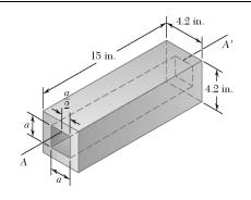
A square hole is centered in and extends through the aluminum machine component shown. Determine (a) the value of a for which the mass moment of inertia of the component with respect to the axis AA', which bisects the top surface of the hole, is maximum, (b) the corresponding values of the mass moment of inertia and the radius of gyration with respect to the axis AA'. (The specific weight of aluminum is  $0.100 \text{ lb/in}^3$ .)
