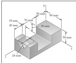
Determine the mass products of inertia  $I_{xy}$ ,  $I_{yz}$ , and  $I_{zx}$  of the steel fixture shown. (The density of steel is  $7850 \text{ kg/m}^3$ .)
