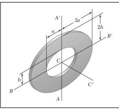
The elliptical ring shown was cut from a thin, uniform plate. Denoting the mass of the ring by m, determine its mass moment of inertia with respect to (a) the centroidal axis BB', (b) the centroidal axis CC' that is perpendicular to the plane of the ring.
