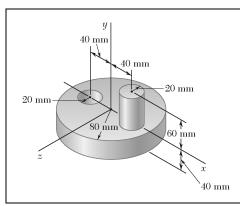
The machine element shown is fabricated from steel. Determine the mass moment of inertia of the assembly with respect to (a) the x axis, (b) the y axis, (c) the z axis. (The density of steel is  $7850 \text{ kg/m}^3$ .)
