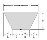
Determine the polar moment of inertia and the polar radius of gyration of the shaded area shown with respect to Point P.
