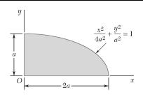
For the quarter ellipse of Problem 9.67, use Mohr's circle to determine the orientation of the principal axes at the origin and the corresponding values of the moments of inertia.
