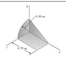
A 2-mm thick piece of sheet steel is cut and bent into the machine component shown. Knowing that the density of steel is 7850 kg/m³, determine the mass moment of inertia of the component with respect to each of the coordinate axes.
