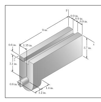
Determine the mass moment of inertia of the steel machine element shown with respect to the y axis. (The specific weight of steel is 490 lb/ft<sup>3</sup>.)
