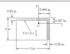
For the angle cross section indicated, determine the orientation of the principal axes at the origin and the corresponding values of the moments of inertia.
