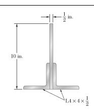
Two L4  $\times$  4  $\times$   $\frac{1}{2}$  -in. angles are welded to a steel plate as shown. Determine the moments of inertia of the combined section with respect to centroidal axes respectively parallel and perpendicular to the plate.
