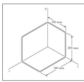
The figure shown is formed of 1.5-mm-diameter aluminum wire. Knowing that the density of aluminum is 2800 kg/m<sup>3</sup>, determine the mass products of inertia  $I_{xy}$ ,  $I_{yz}$ , and  $I_{zx}$  of the wire figure.
