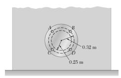
The cover for a 0.5-m-diameter access hole in a water storage tank is attached to the tank with four equally spaced bolts as shown. Determine the additional force on each bolt due to the water pressure when the center of the cover is located 1.4 m below the water surface.
