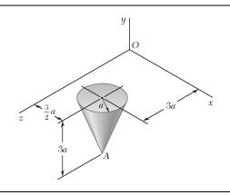
The homogeneous circular cone shown has a mass m. Determine the mass moment of inertia of the cone with respect to the line joining the origin O and Point A.
