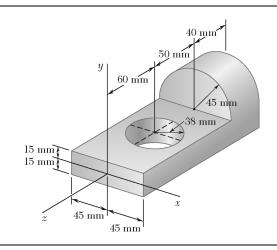
Determine the mass moment of inertia and the radius of gyration of the steel machine element shown with respect to the x axis. (The density of steel is  $7850 \text{ kg/m}^3$ .)
