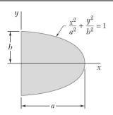
Determine the moment of inertia and the radius of gyration of the shaded area shown with respect to the x axis.
