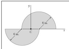
Using Mohr's circle, determine the moments of inertia and the product of inertia of the area of Problem 9.73 with respect to new centroidal axes obtained by rotating the x and y axes  $60^{\circ}$  counterclockwise.
