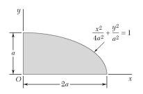
Using Mohr's circle, determine for the quarter ellipse of Problem 9.67 the moments of inertia and the product of inertia with respect to new axes obtained by rotating the x and y axes about O(a) through  $45^{\circ}$  counterclockwise, (b) through  $30^{\circ}$  clockwise.
