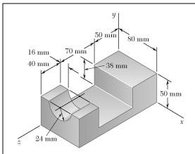
Determine the mass moment of inertia of the steel fixture of Problems 9.145 and 9.149 with respect to the axis through the origin that forms equal angles with the x, y, and z axes.
