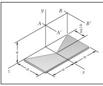
A piece of thin, uniform sheet metal is cut to form the machine component shown. Denoting the mass of the component by m, determine its mass moment of inertia with respect to (a) the axis AA', (b) the axis BB', where the AA' and BB' axes are parallel to the x axis and lie in a plane parallel to and at a distance a above the xz plane.
