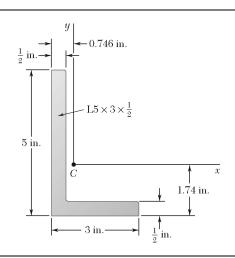
Using the parallel-axis theorem, determine the product of inertia of the L5  $\times$  3  $\times$   $\frac{1}{2}$ -in. angle cross section shown with respect to the centroidal x and y axes.
