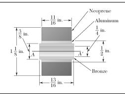
Shown is the cross section of an idler roller. Determine its mass moment of inertia and its radius of gyration with respect to the axis AA'. (The specific weight of bronze is 0.310 lb/in<sup>3</sup>; of aluminum, 0.100 lb/in<sup>3</sup>; and of neoprene, 0.0452 lb/in<sup>3</sup>.)
