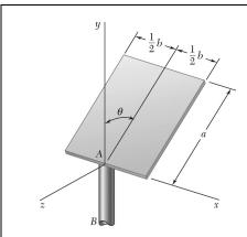
A thin rectangular plate of mass m is welded to a vertical shaft AB as shown. Knowing that the plate forms an angle  $\theta$  with the y axis, determine by direct integration the mass moment of inertia of the plate with respect to (a) the y axis, (b) the z axis.
