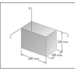
A section of sheet steel 2 mm thick is cut and bent into the machine component shown. Knowing that the density of steel is 7850 kg/m<sup>3</sup>, determine the mass products of inertia  $I_{xy}$ ,  $I_{yz}$ , and  $I_{zx}$  of the component.
