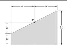
Determine the polar moment of inertia and the polar radius of gyration of the shaded area shown with respect to Point P.
