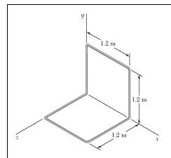
A homogeneous wire with a mass per unit length of 0.056 kg/m is used to form the figure shown. Determine the mass moment of inertia of the wire with respect to each of the coordinate axes.
