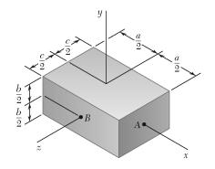
For the rectangular prism shown, determine the values of the ratios b/a and c/a so that the ellipsoid of inertia of the prism is a sphere when computed (a) at Point A, (b) at Point B.
