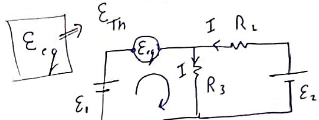
$$I = \frac{E_2}{R_2 + R_3} = \frac{6}{3.3 + 6.2} = 0.626 \text{ mA}$$
