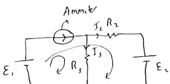
$$\text{small loop: } E_1 - I_3 R_3 = 0$$
