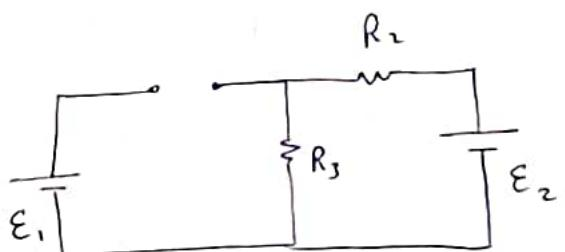
$$R_{eq} = R_2 // R_3 = 2.15 \text{ k}\Omega$$
