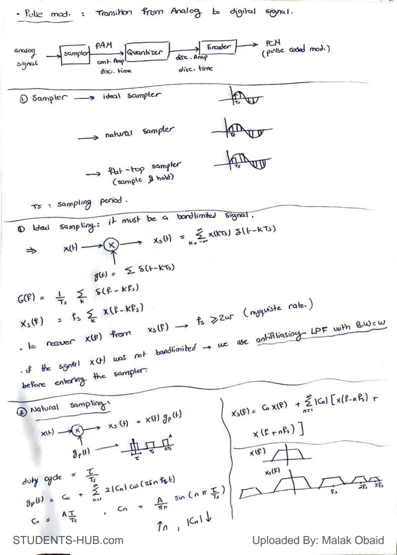
Quantization process: converting cont. Amp. - discrete Amp.
