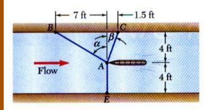
It is desired to determine the drag force at a given speed on a prototype sailboat hull. A model is placed in a test channel and three cables are used to align its bow on the channel centerline. For a given speed, the tension is 40 lb in cable AB and 60 lb in cable AE.
