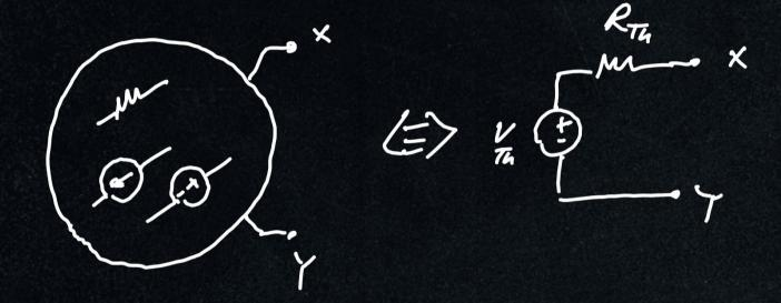
step 1: ca/culate the open circuit voltage across the terminals x4
