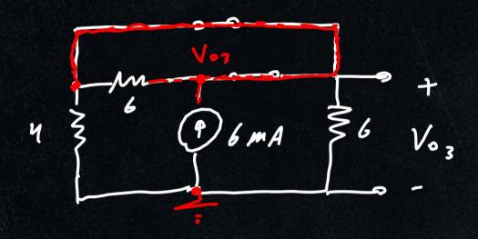
$$-6 + \frac{V_{03}}{4} + \frac{V_{03}}{2} = 6$$
