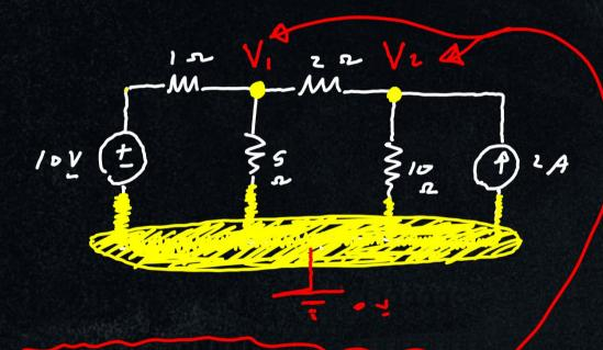
Step 3: Define the node Voltages on the circuit step 1: Determine elle number of essential nodes, ne.
