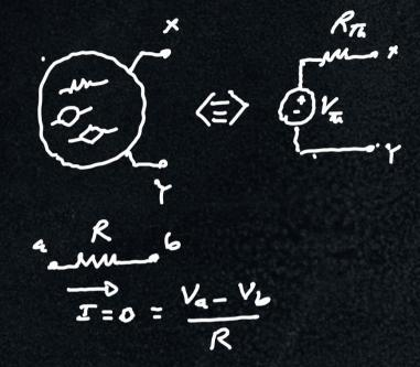
step 2: calculate the short circuit current between the terminals X4Y.
