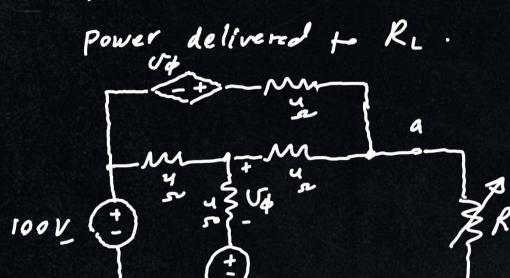
Find the Value of RL to enable the circuit to deliver maximum power and Kind the maximum power delivered to RL = RTH VT6 = 4I + Vp + 20
