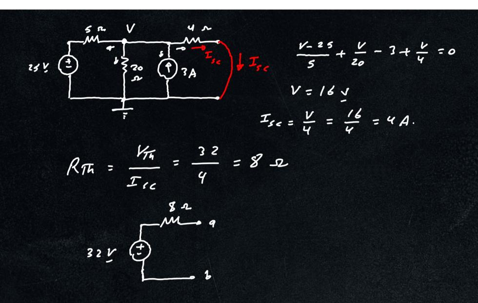
Method 2:- It is useful if the network contains only indep, sources and resistors
