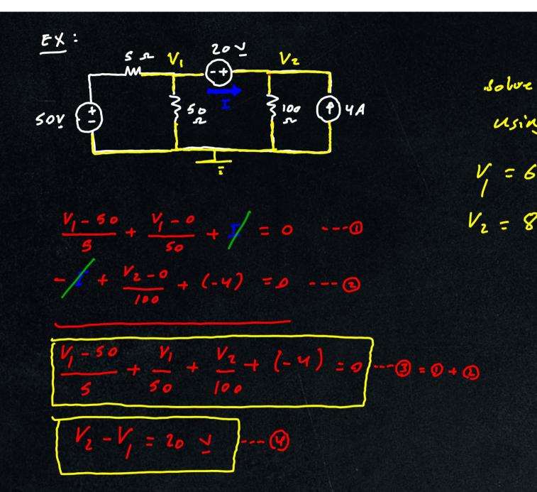
When a voltage source is between two assential modes, we can combine these modes to form a super-mode.
