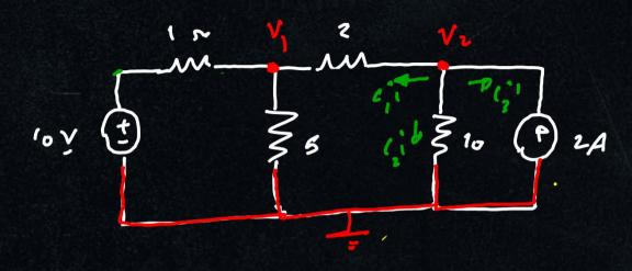
$$\begin{cases} V_{2} - V_{1} \\ \frac{1}{2} \\ \end{pmatrix} + \left( \frac{V_{2} - o}{1o} \right) + (-2) = 0 \qquad (2)$$
