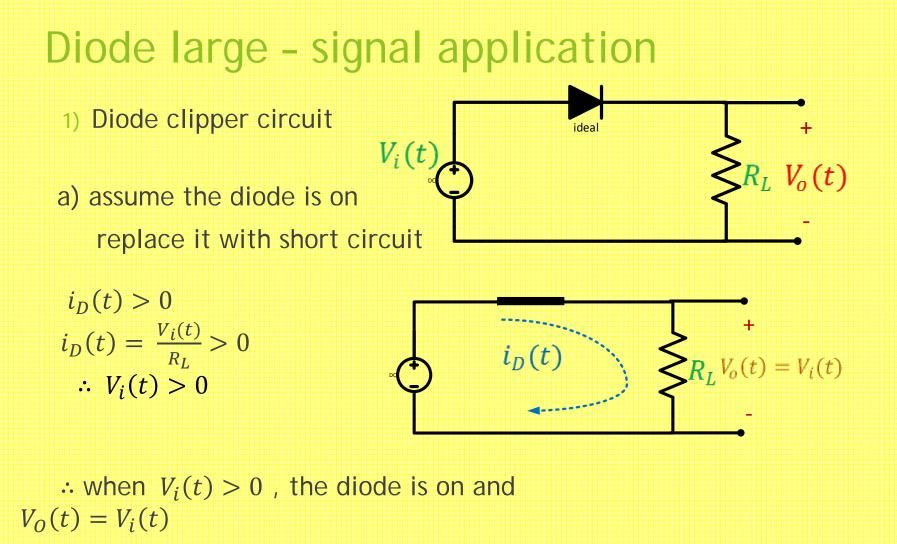
$\therefore$  when  $V_i(t) < 0$ , the diode is off and  $V_0(t) = 0$ .
