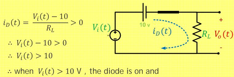
$$V_{0}(t) = V_{i} - 10$$
