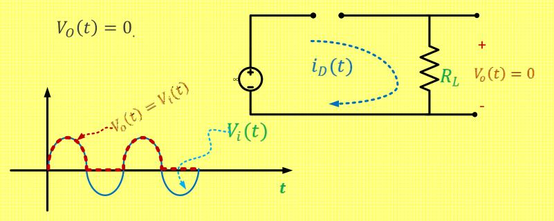
.. the clipper circuit used to eliminate portion of the input signal .
