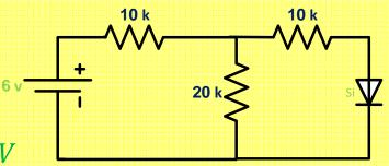
assume the diode is on , replace it with  $V_K = 0.7 V$
