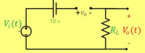
: when  $V_i(t) < 10$  V, the diode is off and  $V_O(t) = 0$
