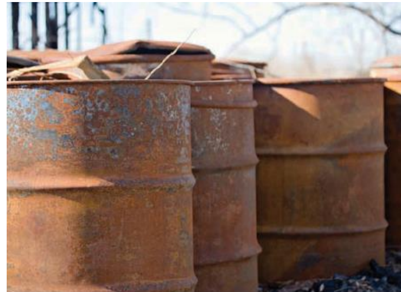
FIGURE 5.8 Iron reacts with oxygen to form iron oxide as seen on these rusted barrels. (Photo by Steven Robertson/iStockphoto)
