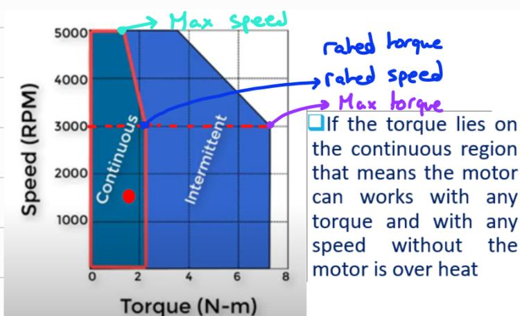
\* If the torque-speed point lies in the intermittent region, the motor can work for 3 seconds or a little longer and provide  $T = 3T_{rated}$  (peak torque)
