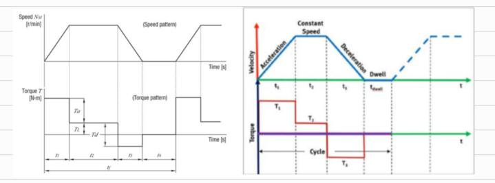
$$(T_{rms})^2 = T_1^2 t_1 + T_2^2 t_2 + T_3^2 t_3 + \dots + T_n^2 t_n$$
