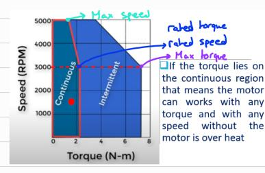
\* If the torque - speed point lies in the intermittent region, the motor can work for 3 seconds or a little longer and provide T= 3 Trated (peak torque)
