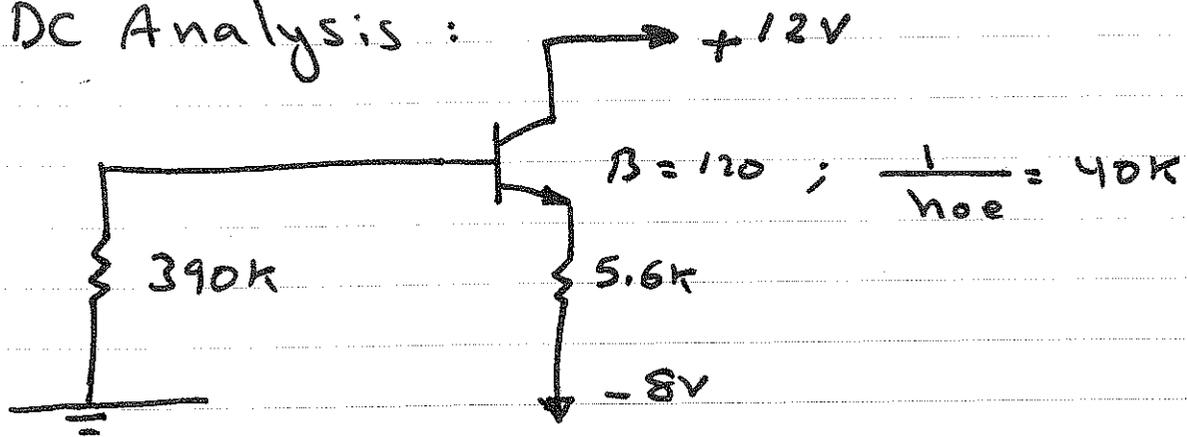
$$390k I_B + V_{BE} + 5.6k I_E - 8 = 0$$
