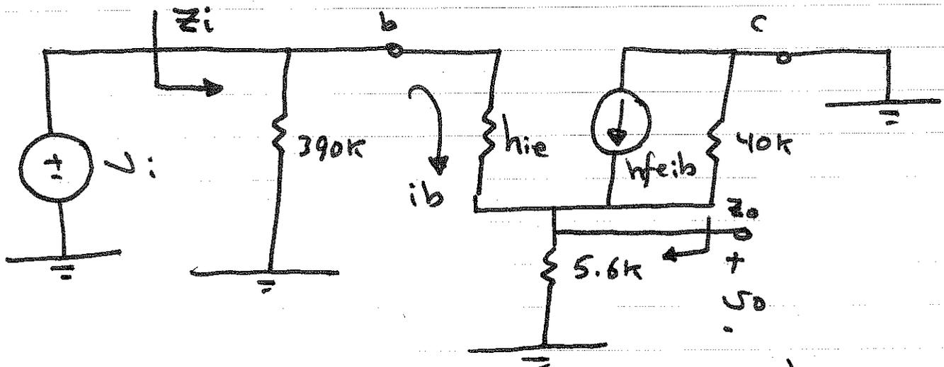
$$Z_i = 390k \parallel \left( h_{ie} + (5.6k \parallel 40k)(h_{fe} + 1) \right) = 236k$$
