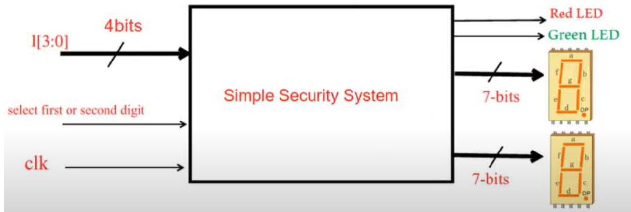
Figure 9.2: High level view of the system.
