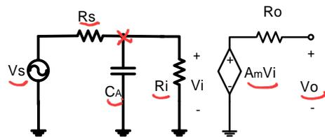
$$\rightarrow |A(j\omega)| = A_v(\text{mid}) \frac{1}{\sqrt{1 + [\omega C_A (R_s // R_i)]^2}}$$
