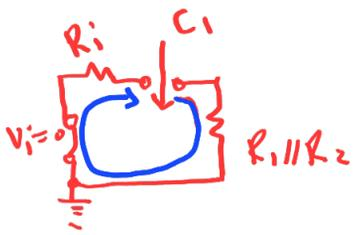
$R_{th1} \text{ seen by } C_1 = (R_1 || R_2) + R_i$
