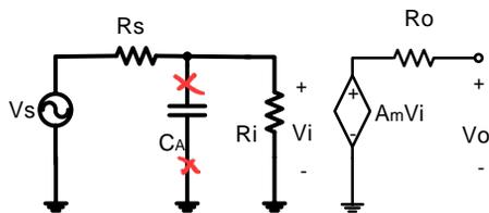
$$\rightarrow \omega_H C_A (R_s // R_i) = 1$$
