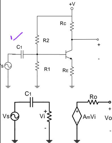
$$|A(j\omega)| = \frac{A_m R_i}{\sqrt{(R_i)^2 + \left(\frac{1}{\omega C_1}\right)^2}}$$
