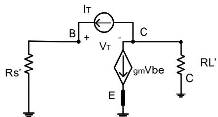
$$RL'(I_T + g_m V_{be}) + I_T R_s' = V_T$$
