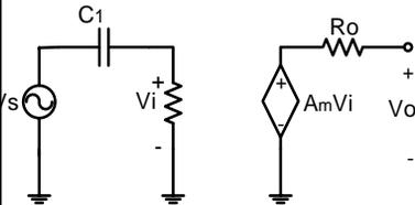
$$A(j\omega) = A_m \left( \frac{1}{1 + \left( \frac{\omega_{c1}}{j\omega} \right)} \right) \left( \frac{1}{1 + \left( \frac{\omega_{c2}}{j\omega} \right)} \right)$$
