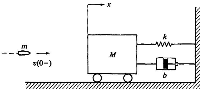
Figure 4–14 Mechanical system subjected to an impulse input.
