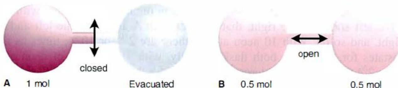
Figure 20.1 Spontaneous expansion of a gas The container consists of two identical flasks connected by a stopcock. A, With the stopcock closed, 1 mol of neon gas occupies one flask, and the other is evacuated. B, Open the stopcock, and the gas expands spontaneously until each flask contains 0.5 mol.
