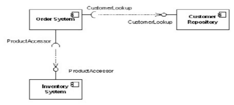
showing a component's relationship with other components, the lollipop and socket notation must also include a dependency arrow (as used in the class diagram). On a component diagram with lollipops and sockets, note that the dependency arrow comes out of the consuming (requiring) socket and its arrow head connects with the provider's lollipop
