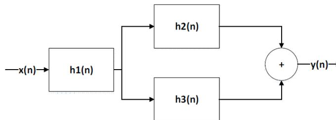
$$h_1[n] = \delta[n - 2], h_2[n] = \left(\frac{2}{5}\right)^n u[n], \text{ and } h_3[n] = 2\delta[n].$$
