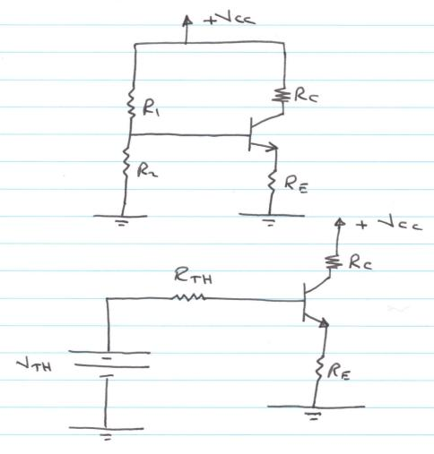
$$\sqrt{TH} = \frac{R_2}{R_1 + R_2} \sqrt{cc}$$
