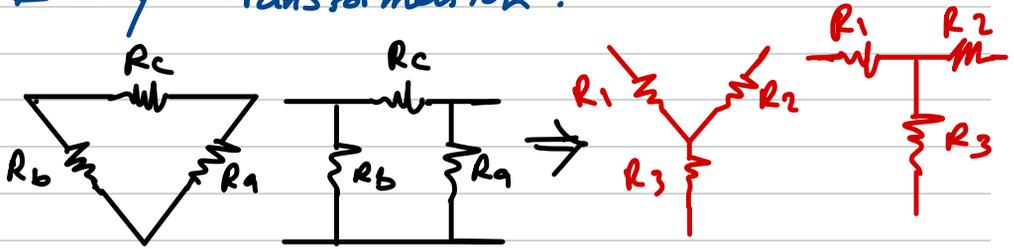
$$R_1 = \frac{R_b R_c}{R_a + R_b + R_c}, \quad R_2 = \frac{R_a R_c}{R_a + R_b + R_c}, \quad R_3 = \frac{R_a R_b}{R_a + R_b + R_c}$$
