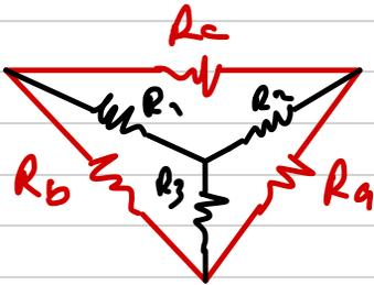
$$R_a = \frac{R_1 R_2 + R_2 R_3 + R_1 R_3}{R_1}$$
