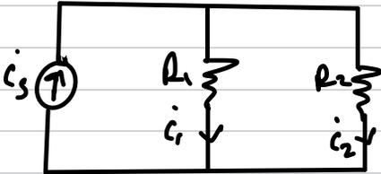
$$i_1 = \frac{i_s R_2}{R_1 + R_2}$$
