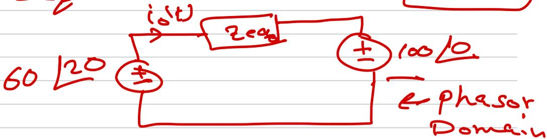
$$i_o(t) = \frac{60 \angle 20^\circ - 100 \angle 0^\circ}{2 + j} \leftarrow \begin{array}{l} \text{Polar} \\ \text{Rect} \end{array}$$
