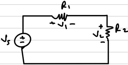
$$V_1 = \frac{V_s R_1}{R_1 + R_2}$$
