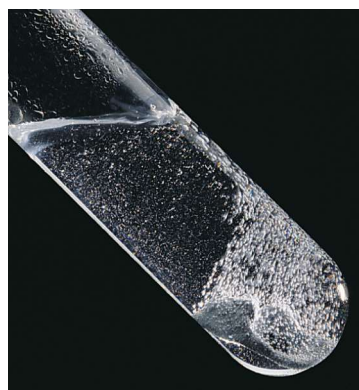
Figure 4.14 The displacement of \text{H}_2 from acid by nickel.
