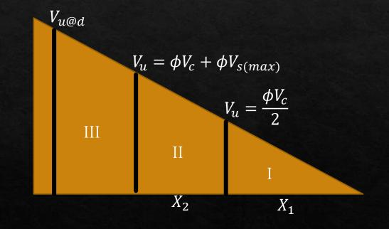
♦ Calculate the shear force the section can support with max spacing and locate it on the shear diagram
