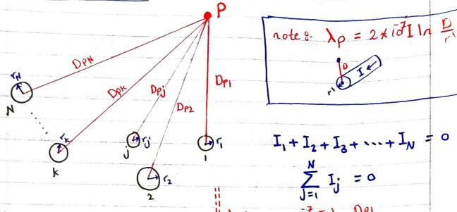
λκρ→ Flux linkages for the conductor k up to a point p due to the currents flowing in conductors 1,2,.... N.
