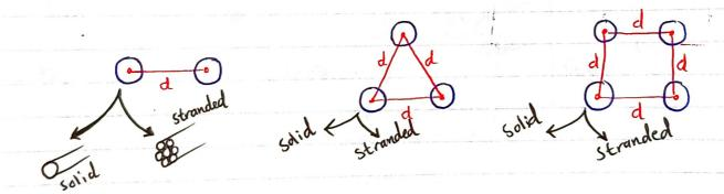
>> Extra-high voltage transmission lines are usually constructed with bundled conductors. Bundling reduces the line reactance, which improves the line performance and increase the power capability at the line. Bundling also reduces the voltage surface gradient, which in turn reduces Corona loss, radio interference, and surge impedance. (\frac{1}{5})
