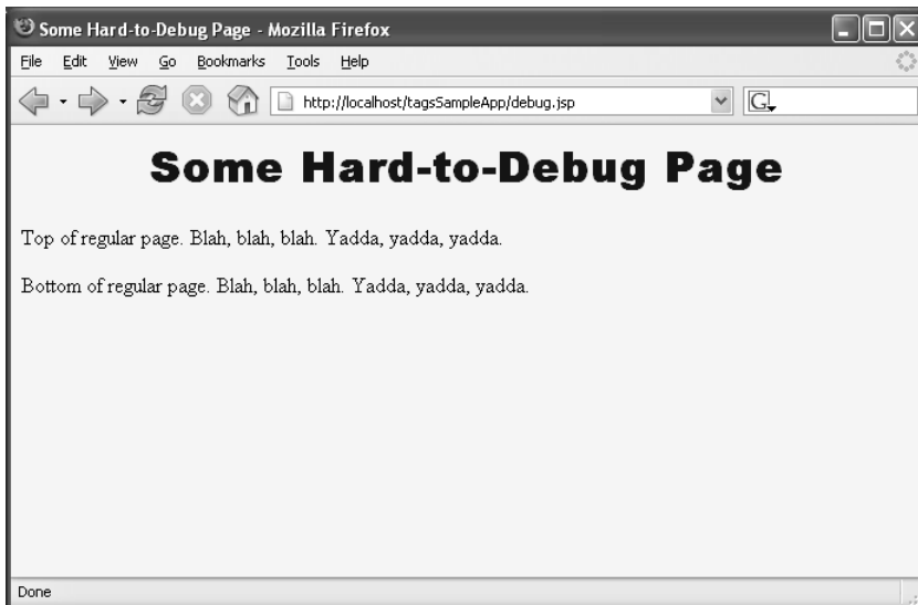
Figure 7-4 Result of debug.jsp page without supplying the debug request parameter.
