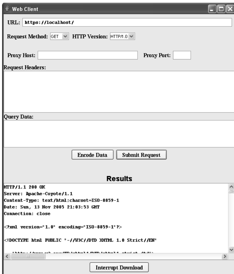
Figure 3-41 Test of SSL connection to Apache Tomcat, https://localhost/ . When starting WebClient, command-line system properties specify information about the Root CA (for the returned SSL server certificate).
