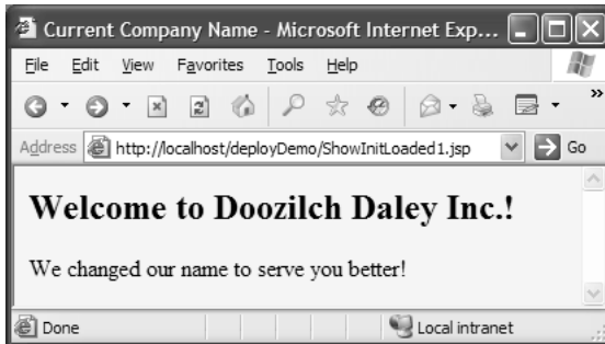
Figure 2-16 Result of invoking http://localhost/deployDemo/ShowInitLoaded1.jsp . This page retrieves the name of the company previously stored in the ServletContext by the LoadInitServlet .
