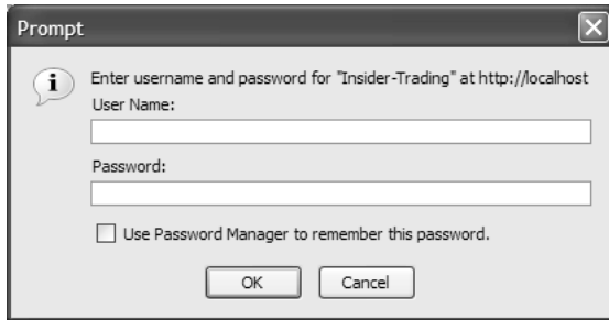
Figure 4–3 When the browser first receives the 401 (Unauthorized) status code, it opens a dialog box to collect the username and password.
