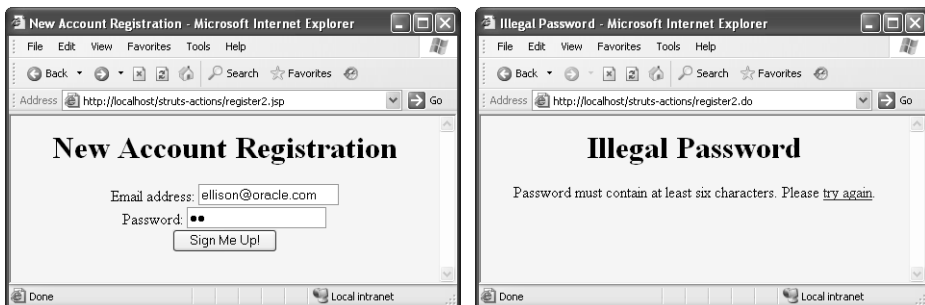
Figure 10–10 Registration form with an illegal password—one that doesn't contain six characters (left). Response for a "bad-password" condition (right).
