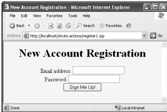
Figure 10–5 Initial registration page. The ACTION submits to register1.do.
