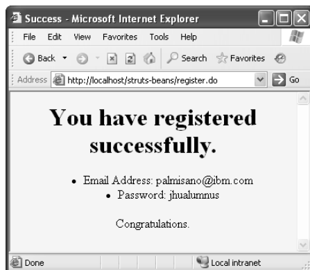
Figure 10–17 Successful registration page displayed to user. The legal address and password, properties of the form bean in the request scope, are displayed in the response page through the bean:write custom tag.
