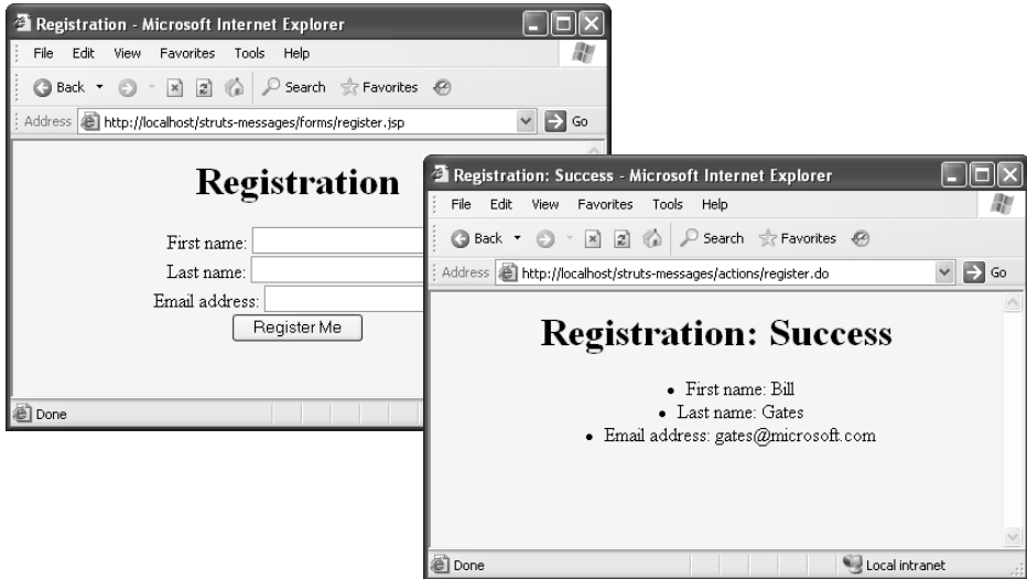
Figure 11-2 Result of struts-message Web application. For both the input page and results page, bean:message retrieves the title, heading, and field labels from the default properties file.
