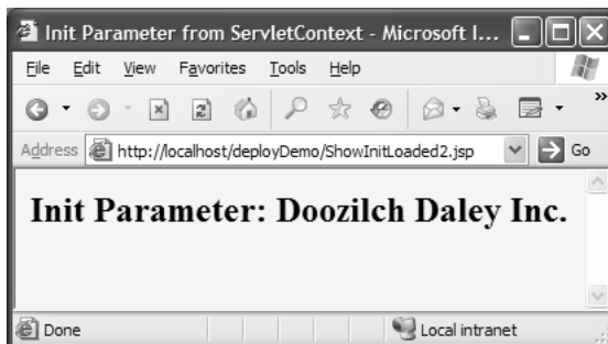
Figure 2-17 Result of invoking http://localhost/deployDemo/ShowInitLoaded2.jsp . This page retrieves the name of the company previously stored in the ServletContext by the LoadInitServlet .
