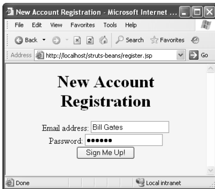
Figure 10–15 Registration form with an illegal e-mail address—doesn't contain an @ symbol (left). Response for a "bad-address" condition (right). The bean:write tag displays both the bad address (from the form bean) and suggested address (from the suggestion bean).
