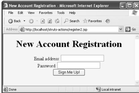
Figure 10–8 Initial registration page. The ACTION submits to register2.do .
