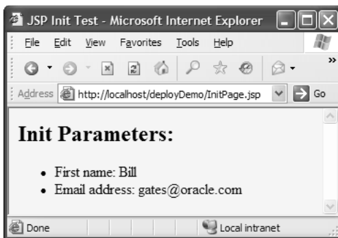
Figure 2–14 Mapping a JSP page’s original URL to the registered custom URL pattern prevents users from accidentally accessing the uninitialized version.
