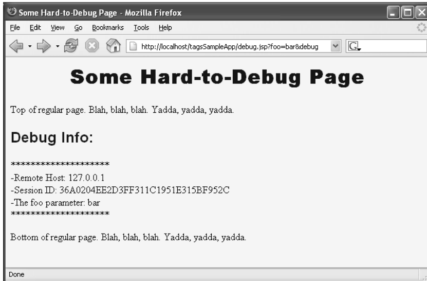
Figure 7–5 Result of debug.jsp page when the debug request parameter is supplied.
