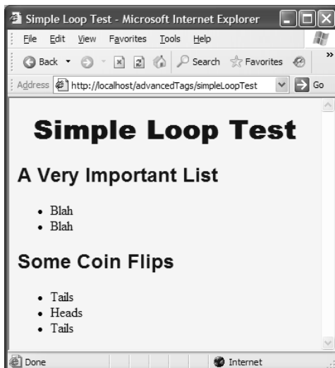
Figure 8-2 Result of simple loop test. The number of times the word “blah” displays, as well as the number of simulated coin flips, is random.
