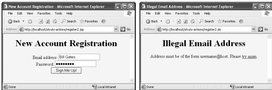
Figure 10–9 Registration form with an illegal e-mail address—one that doesn't contain an @ symbol (left). Response for a "bad-address" condition (right).
