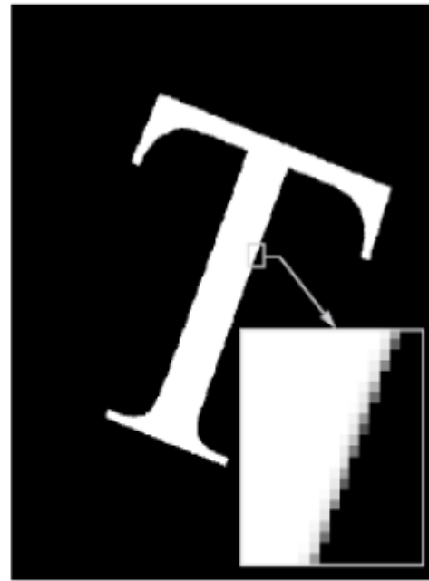
Rotation by 21° using inverse mapping and bicubic interpolation
