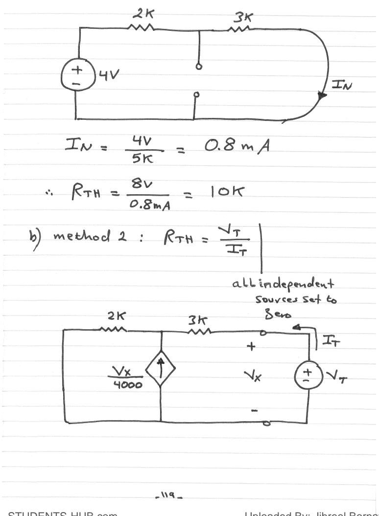
3K I. 4 2kVx + J-T  $\frac{V \times}{2}$ KVL :  $-V_T + 3K I_T + 2K I_T + \frac{1}{2} =$ 0 VX = VT  $\therefore R_{TH} = \frac{V_T}{I_T} = 10 \text{ K}$ -120\_ Uploaded By: Jibreel Bornat STUDENTS-HUB.com
