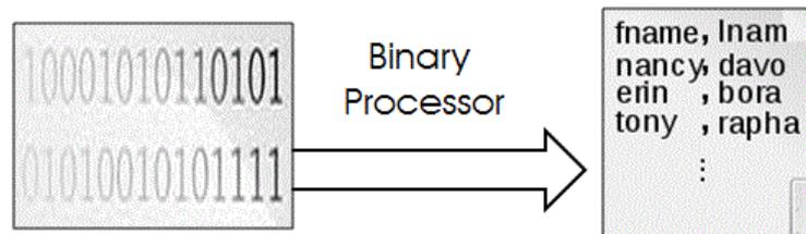
Many programs produce output files that are used as input files for other programs. If there is no need for a human to read the file, it is a waste of computer time for the first program to convert its internal data format to a stream of characters, and then for the second program to have to apply an inverse conversion to extract the intended data from the stream of characters. We can avoid this unnecessary translation by using a binary file rather than a text file.
